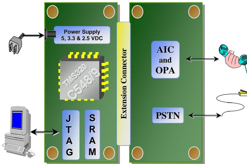
The TMS320C54x generation of the TI TMS320 DSP is fabricated using static CMOS integrated circuit technology. The combination of advanced modified Harvard architecture with one program bus and three data memory buses, additional on-chip peripherals, on-chip data memory, and a highly specialized instruction set is the basis for the operational flexibility and speed of this device.
