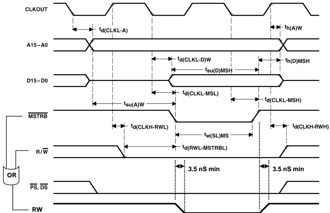
Figure 10. SRAM Write Timing
