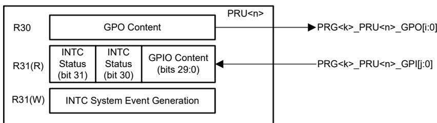
**Figure 2-1. PRU GPIO Interface**
