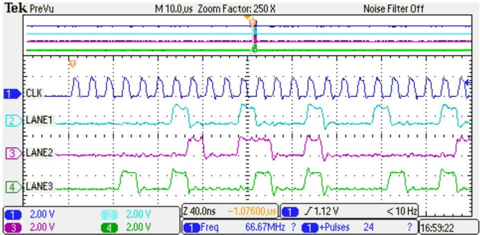
Figure 3-5. 4-Lane Parallel Data Transmission
