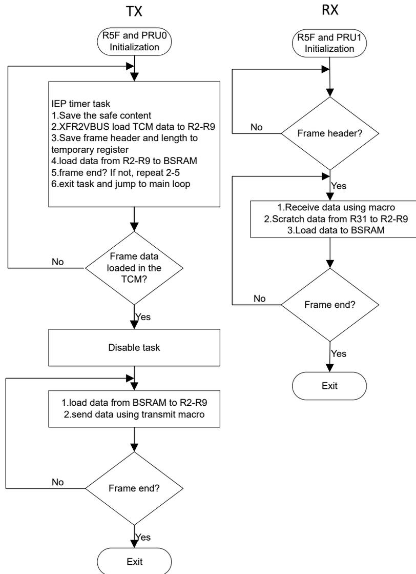
**Figure 2-6. Workflow for GPIO Direct Mode**
