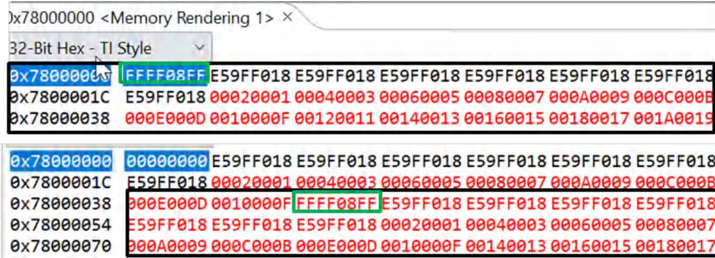
Figure 3-2. Transmit and Receive Data Comparison
