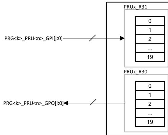
Figure 2-2. PRU Direct Input and Output Mode Block Diagram
