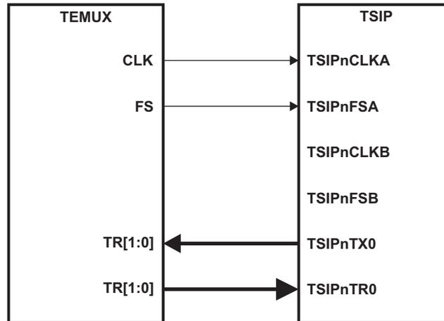
In this configuration, CLKA and FSA are used by the transmit and receive logic for clock and frame synchronization.
