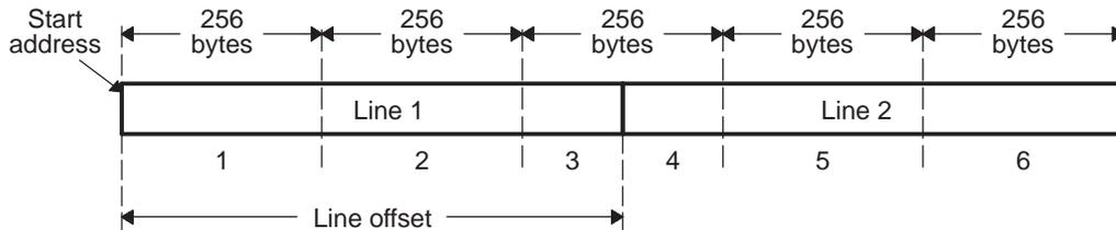
Depending on the width of each line, not programming the starting address and/or line offset registers to be on 256-byte boundaries (32- or 64-byte boundaries are required) may result in more DMA requests. [Figure 49](#) shows two cases of programming the starting address and line offset register.
