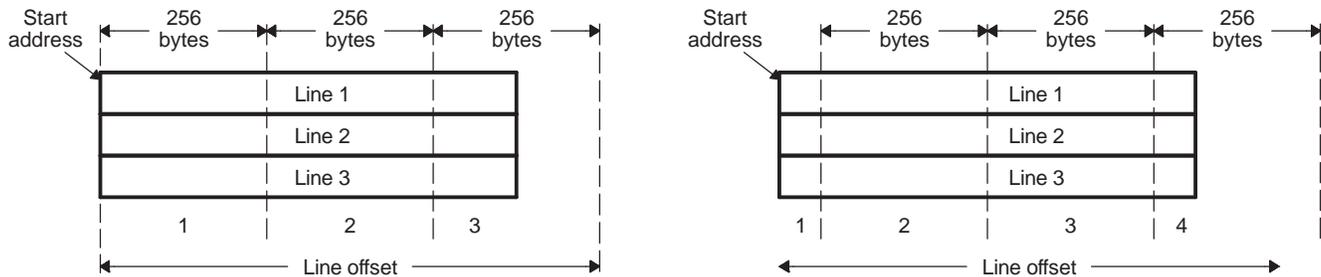
(a) Start address – 256 byte aligned
