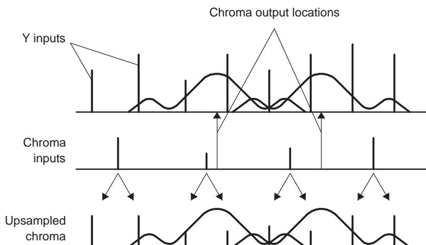
The chroma input values are internally replicated to realize 1:2 upsampling to line up with luma input values. Only required chroma outputs are computed; they correspond to the even luma outputs.
