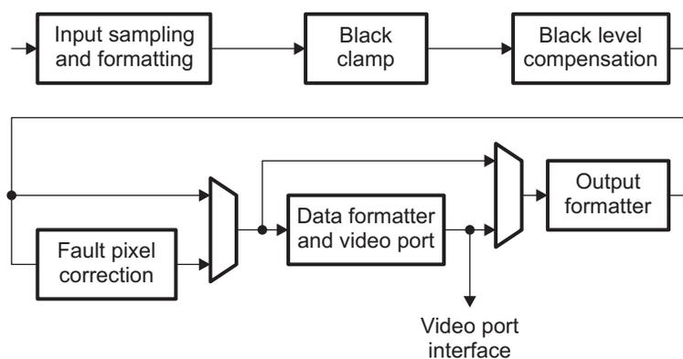
The following sections describes the CCD controller processing for the YUV input modes (SYN\_MODE.INPMODE = 1 or 2 || REC656IF.REC656ON = 1) in more detail. In this mode, YUV422 input data typically at 8-bits per luma/chroma sample is input.
