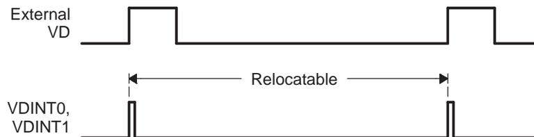
In the case of the SYN\_MODE.VDPOL = 1 ([Figure 56](#)), the VDINT0 and VDINT1 HD counters begin counting HD pulses from the falling edge of the external VD.
