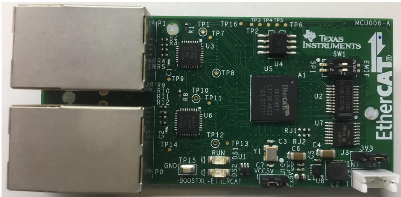
**Figure 2. TMDSECATCNCNCD379D Adapter Board**
