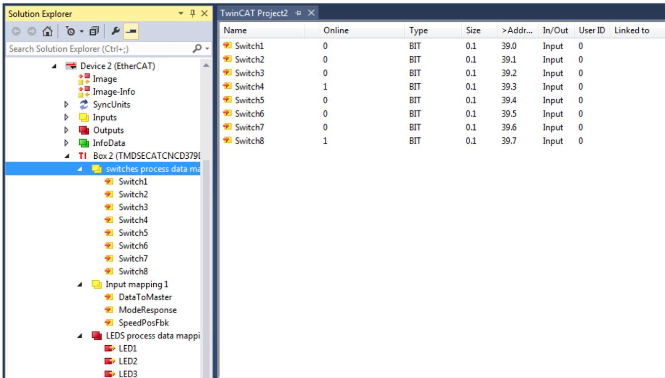
The screenshot shows the TwinCAT Project2 interface. On the left is the Solution Explorer showing a project structure for 'Device 2 (EtherCAT)' with folders for Image, SyncUnits, Inputs, Outputs, InfoData, and a TI Box 2 (TMDSECATCNCD379D) containing switches process data mapping, Input mapping 1, and LEDS process data mapping. On the right is a table listing the switches.
