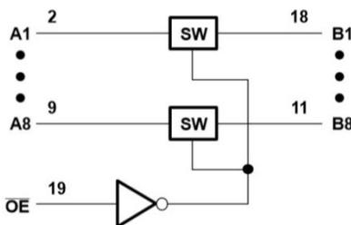
Figure 11. SN74CBTLV3245A Functional Diagram
