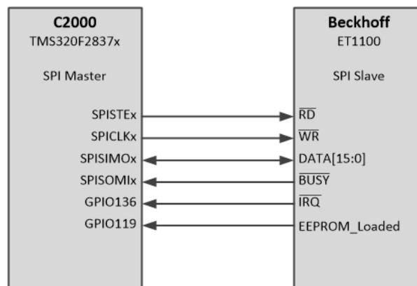
Figure 8. SPI Interface to ET1100 EtherCAT Slave Controller
