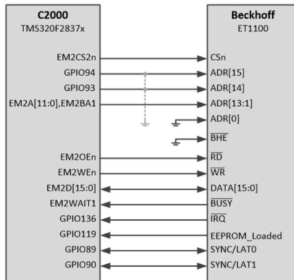
Figure 7. EMIF Interface to ET1100 EtherCAT Slave Controller
