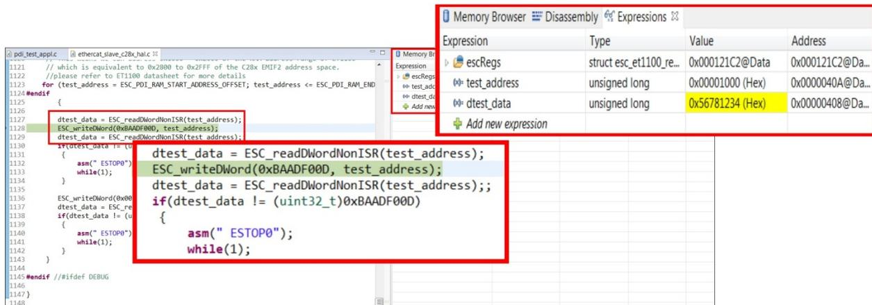
Figure 37. EtherCAT Write to Memory From CCS Project
