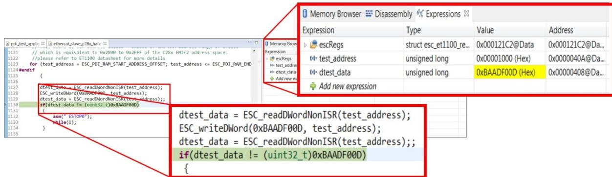
Figure 38. CCS Project Write to EtherCAT Slave
