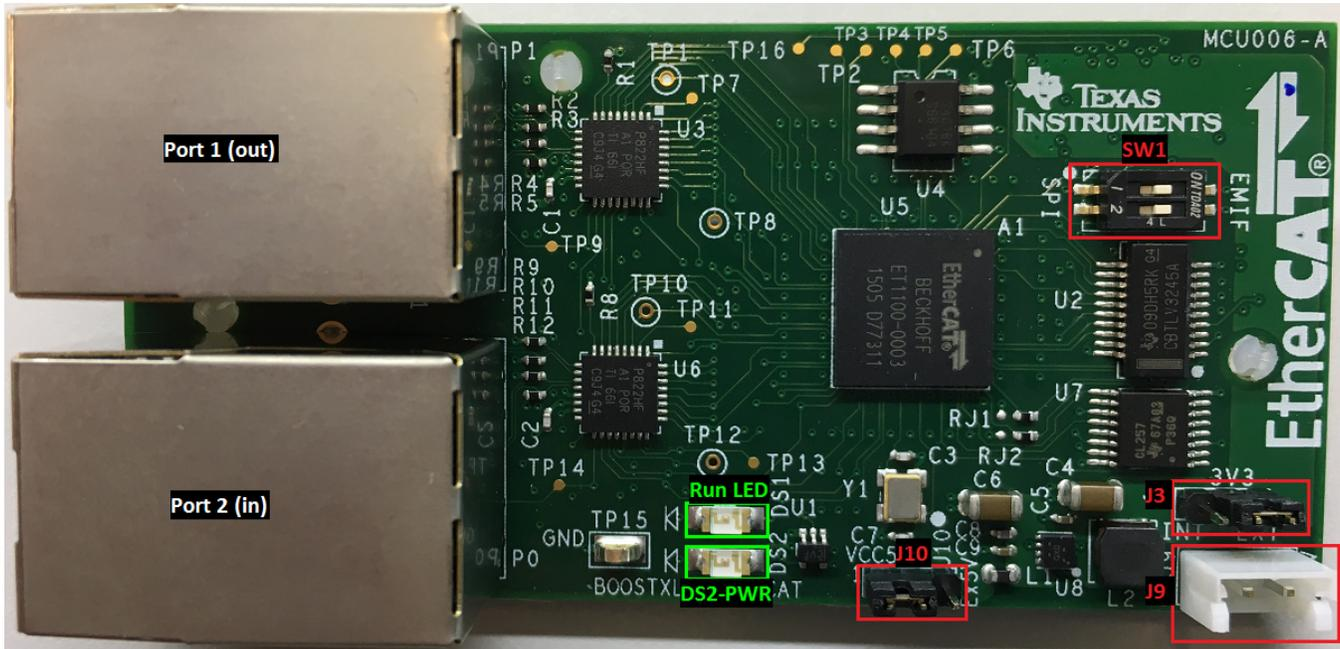
Figure 25. EtherCAT Adapter Board LED and Switch Locations
