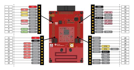
UART (DIO12, DIO13), Reset (LP\_RST) and JTAG (TMS, TCK, TDO and TDI) are also present in the LP-EM Debug Connector. Power (GND, 3V3 and 5V) is also provided.
