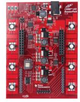
Easily plug in C2000 LaunchPad to the LED BoosterPack to add lighting capability
