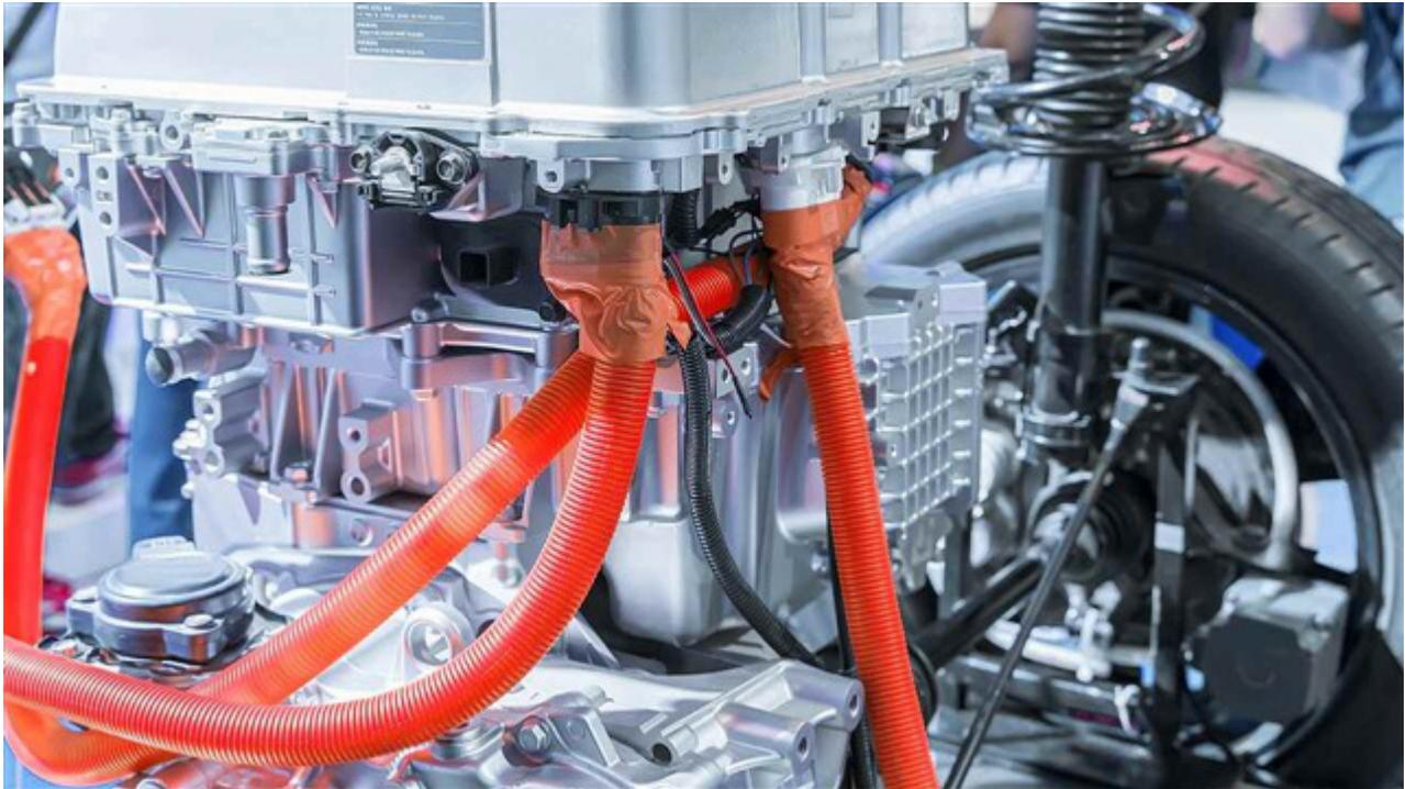
The electric vehicle (EV) traction inverter is the core of the EV. It converts DC from the high-voltage battery to multiphase (usually three-phase) AC to drive the traction motor, and also controls power regeneration from braking. EV electronics are shifting from 400-V to 800-V architectures, which promise:
