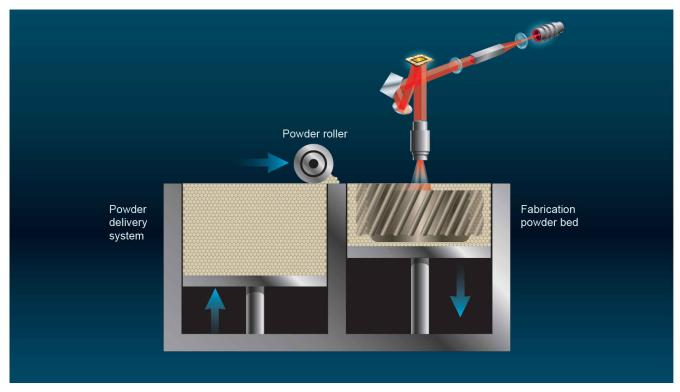
Figure 1. A NIR System Setup Using the DLP650LNIR DMD
