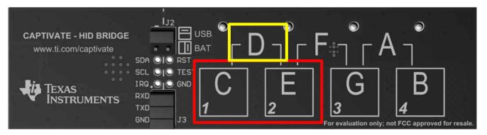
Figure 3. Multi-Touch Output Sound (Yellow) of Both Cap Touch Buttons (Red)
