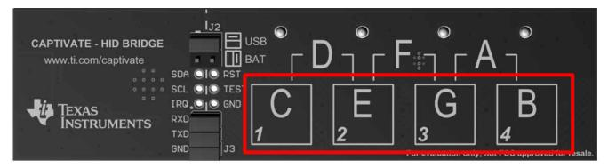
Figure 2. Capacitive Touch Buttons (Red) on CAPMINI Demonstration Board
