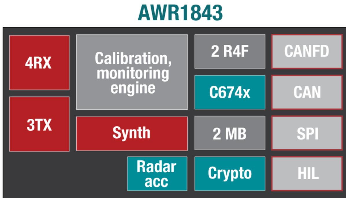
**Figure 2. Components of the AWR1843 Parking Chip.**
