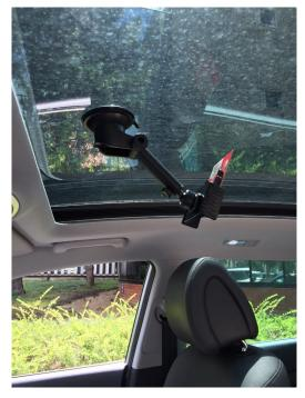
Figure 1. mmWave Sensor Installation on the Sunroof of a Vehicle
