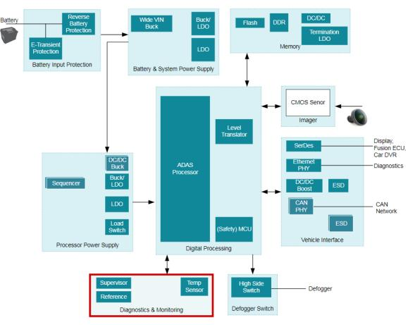
Figure 1. System Block Diagram for a Mono Front Camera
