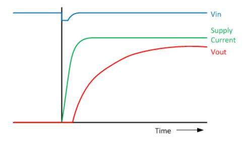
Figure 3. REF2125 Clean-start Example with R<sub>CS</sub> And C<sub>CS</sub>
