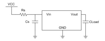
Figure 1. A Precision Voltage Reference Lacking In-rush Current Protection
