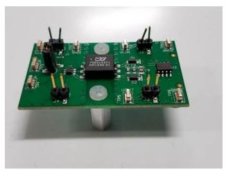
Figure 3. Discrete Solution for Isolated Power with a 4.10mm-thick Isolation Transformer
