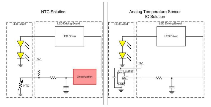
Figure 1. NTC thermistor thermal foldback vs. analog temperature sensor thermal foldback solution
