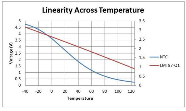
Figure 2. Voltage input to LED driver across temperature
