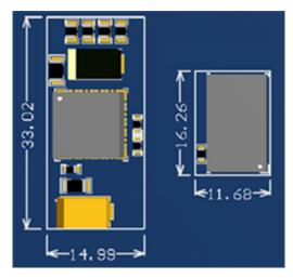
Figure 2. Module Solution Size Can Vary Widely from Module Package Size
