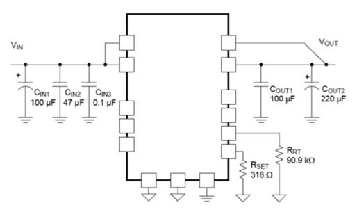
Figure 1. Input and Output Capacitors Add Complexity to Module Circuits
