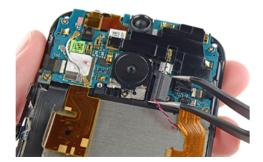
Figure 1. Camera Circuitry in a Smartphone
