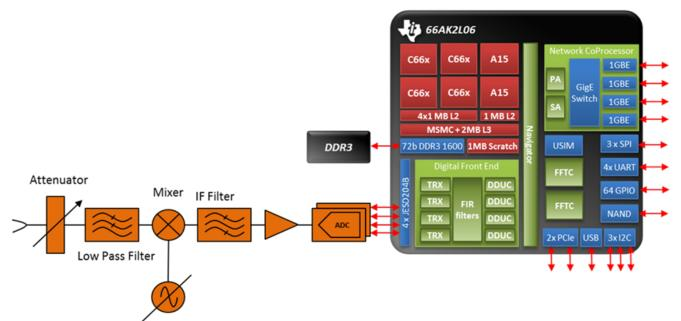
The higher integration, programmability and flexibility offered by the 66AK2L06 SoC translate to significant benefits to customers – C-SWaP (cost, size, weight and power) efficiency and time-to-market acceleration. The combination of DFE and JESD204B eliminates the need for expensive FPGAs/ASICs, further reducing the board space.
