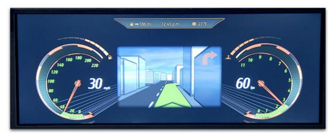
The above describes what we call reconfigurable digital instrument clusters which have virtually endless display possibilities. The "Jacinto 6" family is well suited to power such instrument clusters with its powerful architecture delivering high-level of graphics and robustness with software architecture capable of ASIL-B safety certification. It includes:
