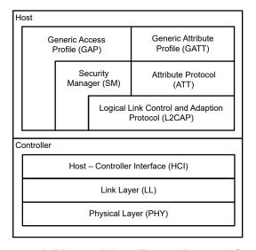
Figure 4-1. Bluetooth Low Energy Protocol Stack
