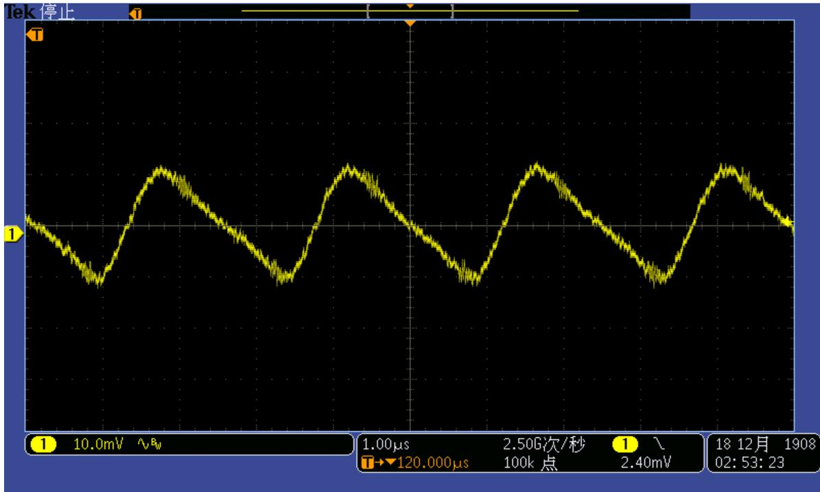
Figure 3-3. Output Voltage Ripple (18 V Channel),  $V_{IN} = 12\text{ V}$
