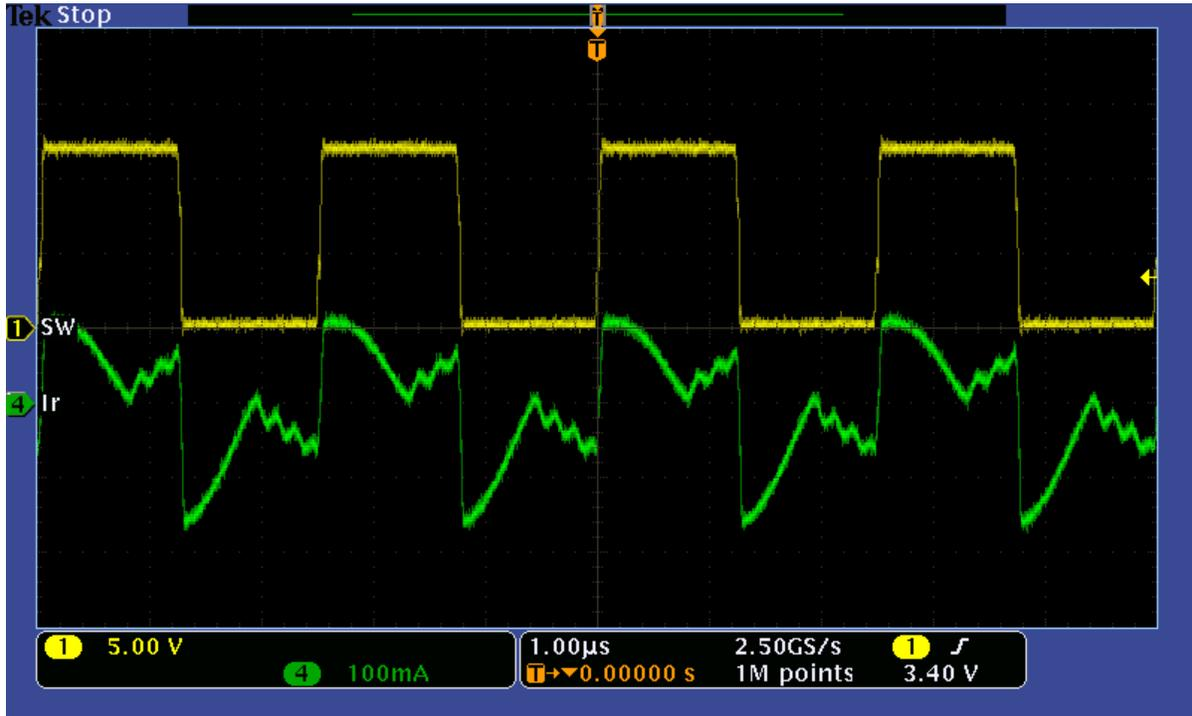
Figure 3-1. Switching , No Load
