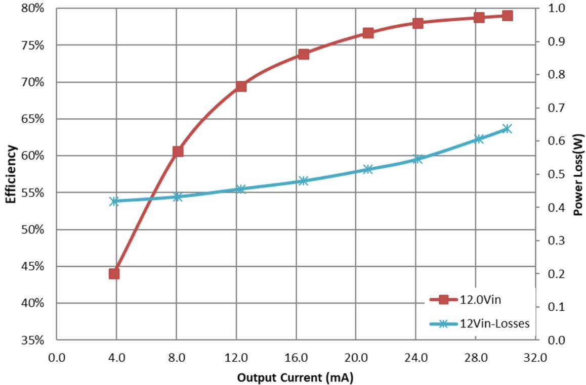
Figure 2-1. Efficiency Graph
