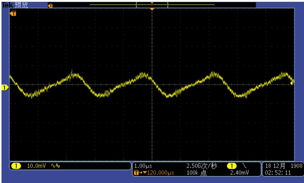
Figure 3-4. Output Voltage Ripple (-2.5 V Channel),  $V_{IN} = 12\text{ V}$
