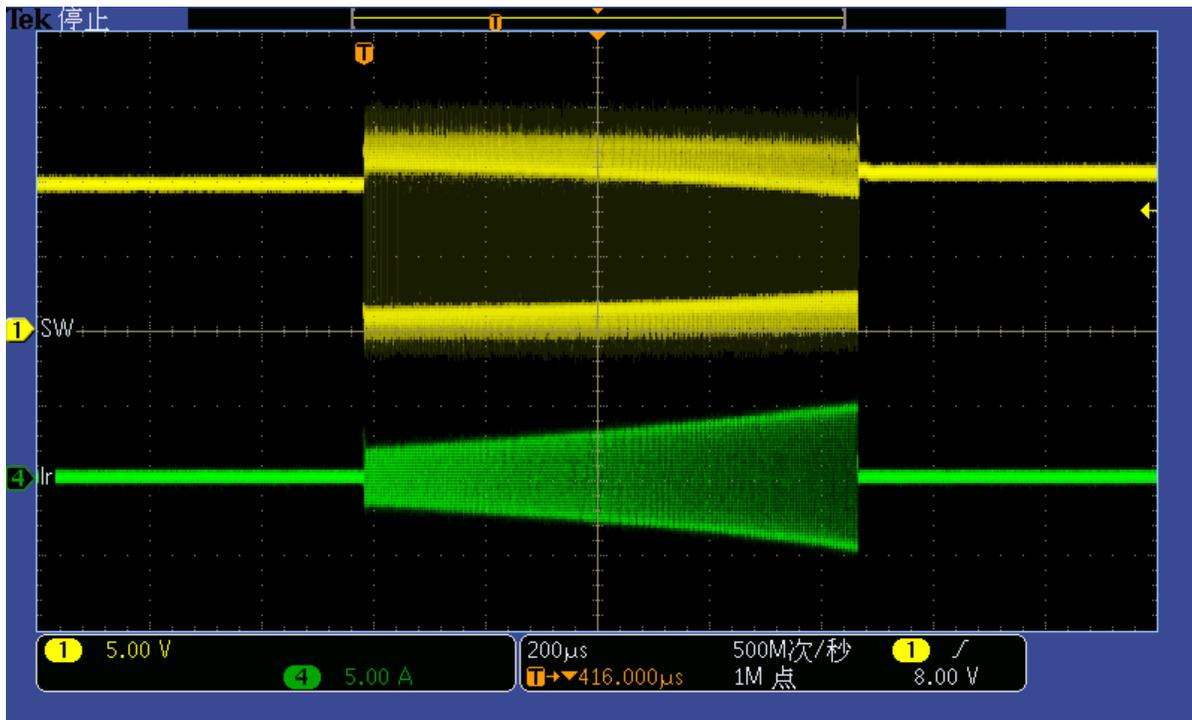
Figure 3-5. Short-Circuit Protection
