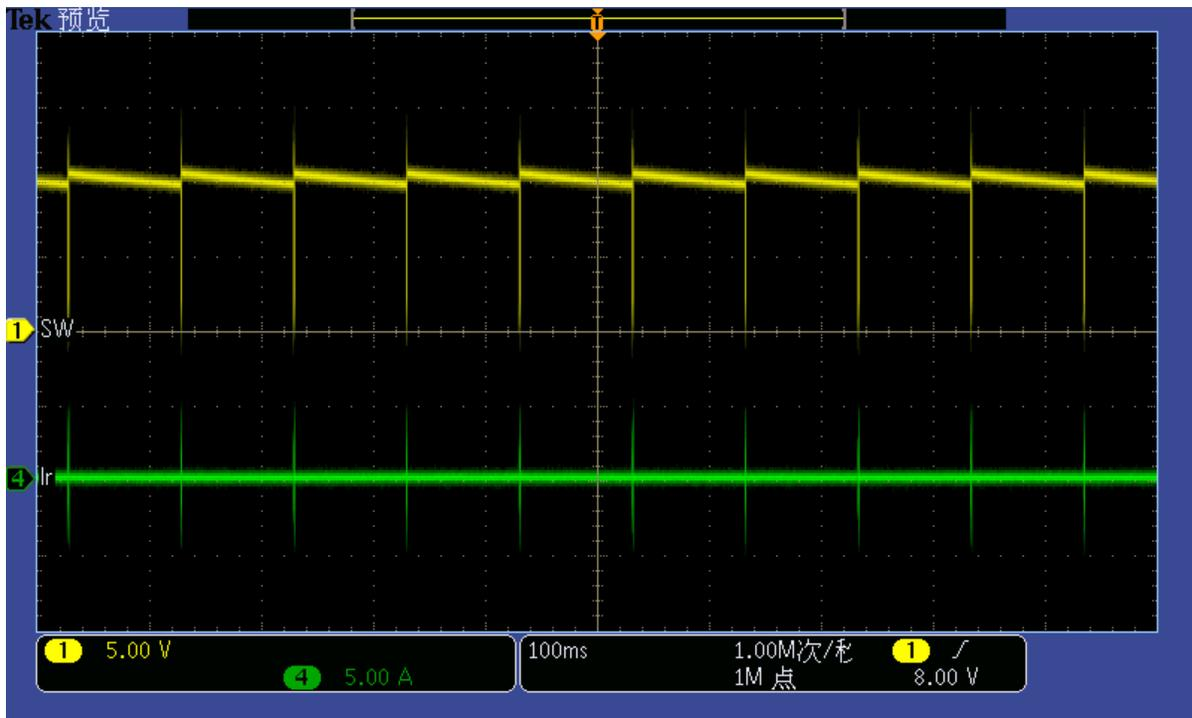
Figure 3-6. Short-Circuit Protection
