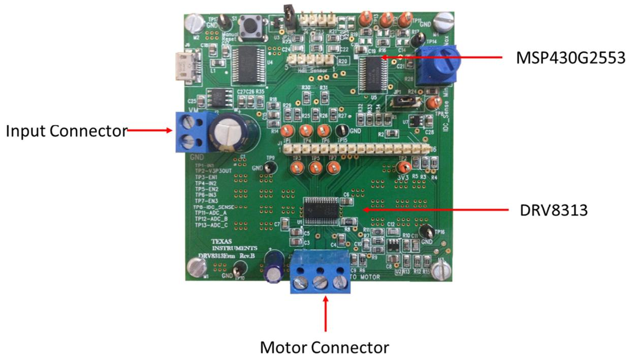
Figure 1: DRV8313 Reference design Circuit Card Assembly
