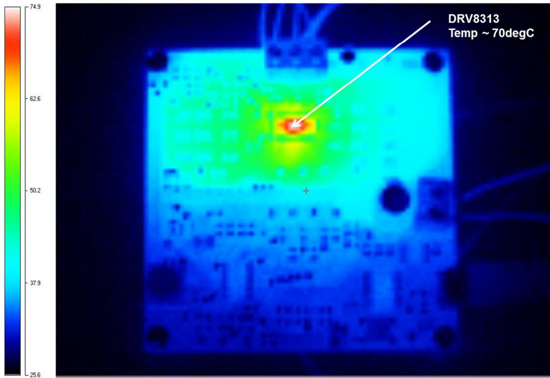
**Figure 6: Thermal image at 48Vdc/0.75Adc, Pin =36Watts**
