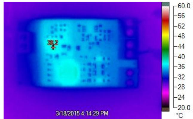
Figure 14. TIDA-00237 Thermal Analysis Full Load,  $V_{IN} = 12\text{ V}$
