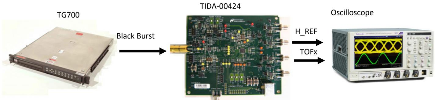
Figure 1. Test setup
