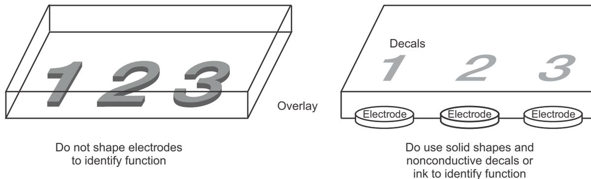
**Figure 10. Button Shape Examples—Dos and Don'ts**
