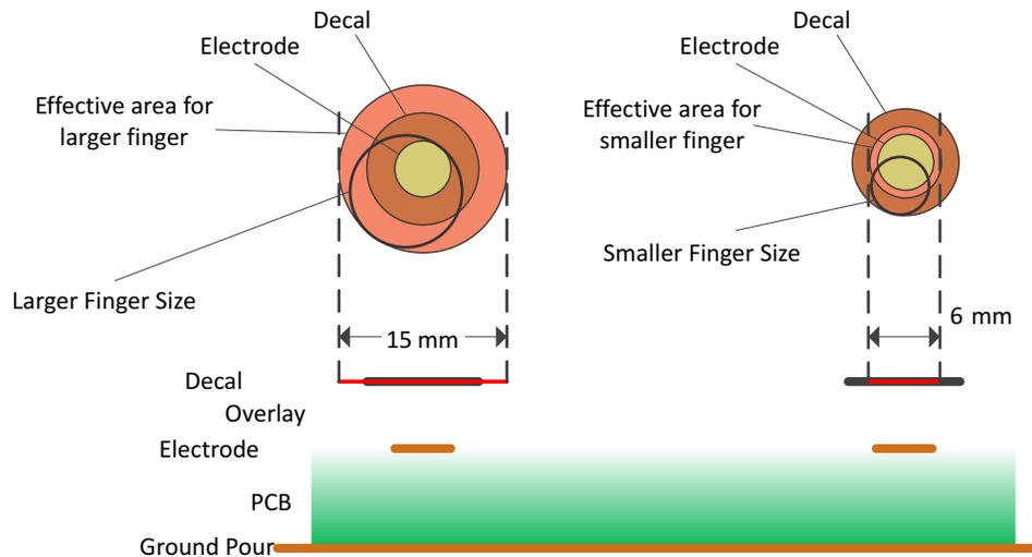
Figure 9. Effective Area Example for Electrode Smaller Than Decal
