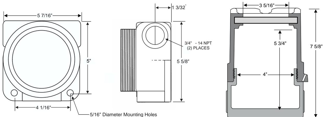
**Figure 2. Explosion-Proof Enclosure (XIHLDGCX From Adalet)**
