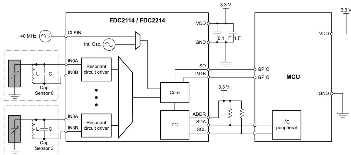
**Figure 12. FDC2114 Simplified Schematic**
