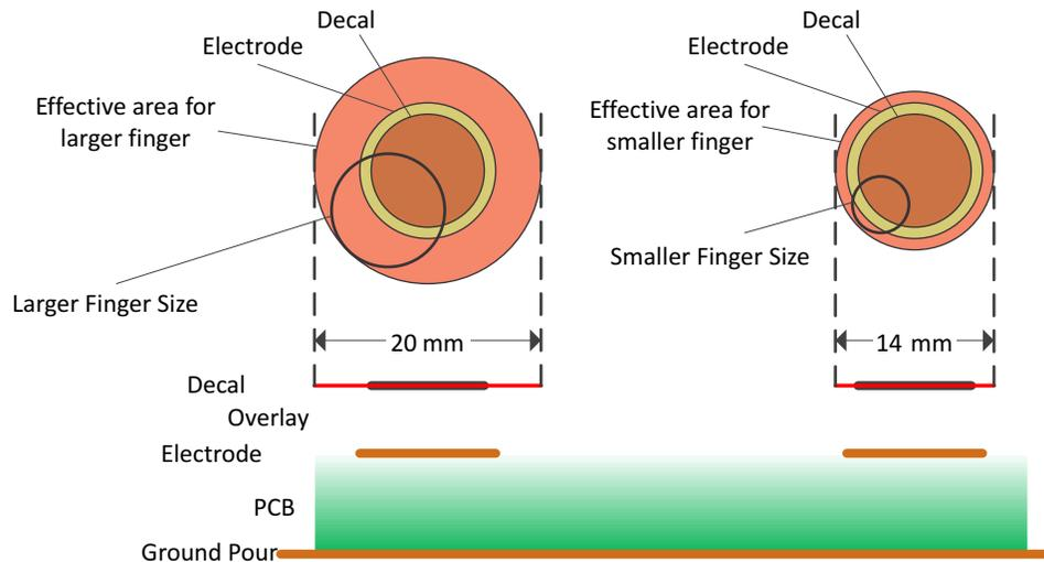
Figure 8. Effective Area Example for Electrodes Larger Than Decal
