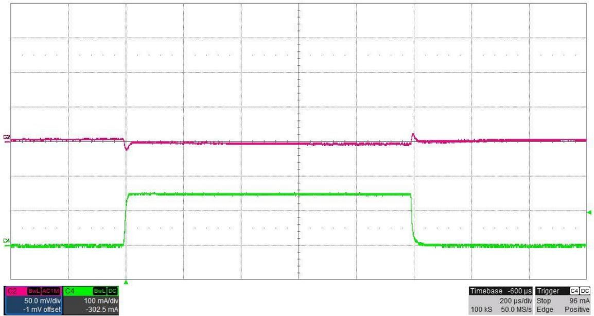
The photo below shows the **15V#2** output voltage (ac coupled) when the load current is stepped between 0A and 0.15A.  $V_{in} = 24V$ .
