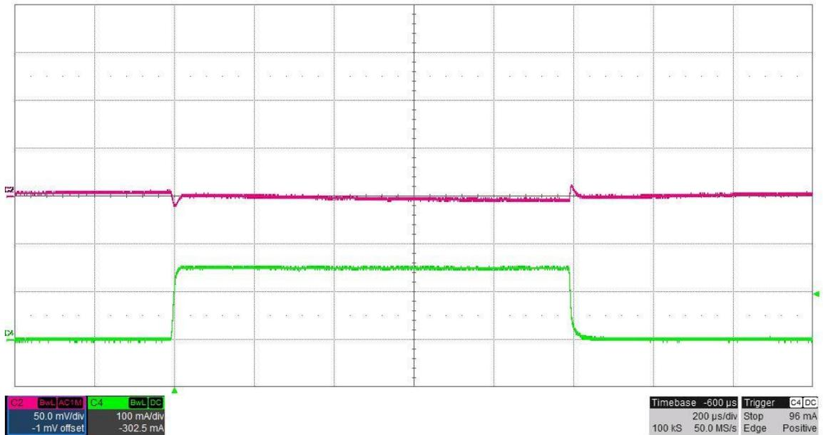
The photo below shows the **5V#2** output voltage (ac coupled) when the load current is stepped between 0A and 0.15A.  $V_{in} = 24V$ .
