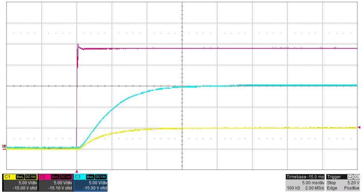
The photo below shows the **15V#2 and 5V#2** output voltage startup waveform, measured at TP16 and TP20, after the input voltage is applied.  $V_{in} = 24V$ ,  $I_{out} = 0.15A$ . (5V/DIV, 5mS/DIV)
