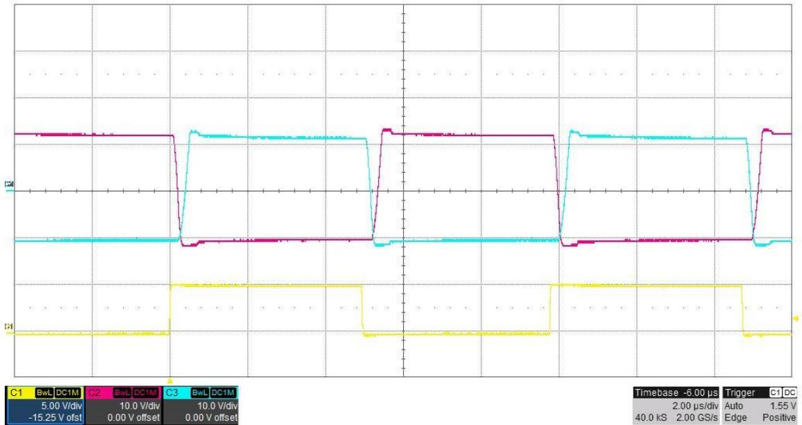
The photo below shows the switch node voltages of **15V#2** and **5V#2**, measured at TP18 and TP25 and the PHASE clock signal. **V<sub>in</sub> = 21.6V**, **I<sub>out</sub> = 0.15A**. (PHASE is 5V/DIV, 10V/DIV, 2uS/DIV)
