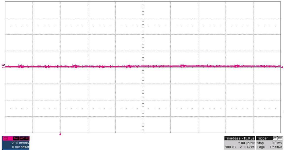
The output ripple voltage is shown in the figure below. The image was taken with the **15V#1** output loaded to **0.15A** and the input voltage set to 26.4V. (20mV/DIV, 5uS/DIV)
