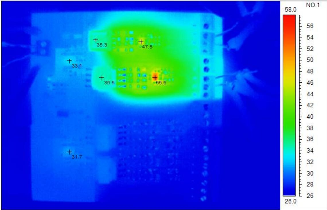
The thermal image below shows the temperature rise with 24Vin and 15V#2 @ 0.15A and 5V#2 @ 0.15A, with no airflow. All other outputs are unloaded.
