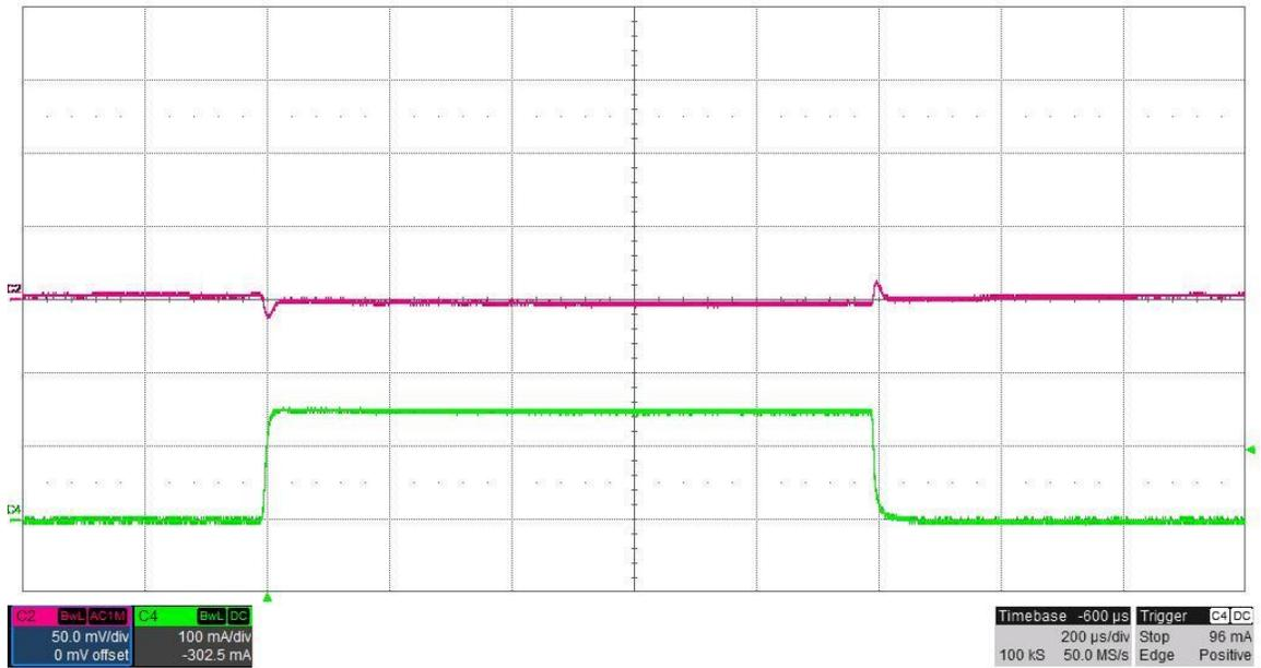
The photo below shows the **15V#1** output voltage (ac coupled) when the load current is stepped between 0A and 0.15A.  $V_{in} = 24V$ .
