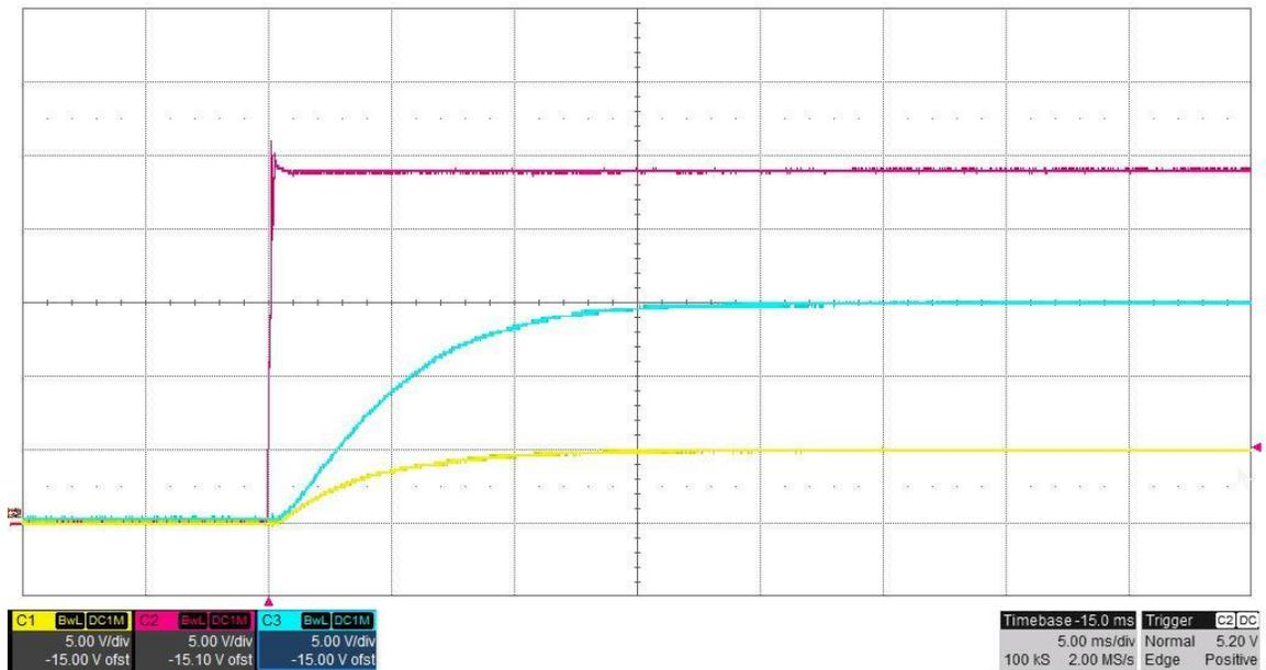
The photo below shows the **15V#2 and 5V#2** output voltage startup waveform, measured at TP16 and TP20, after the input voltage is applied.  $V_{in} = 24V$ ,  $I_{out} = 0A$ . (5V/DIV, 5mS/DIV)
