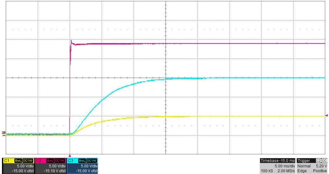
The photo below shows the **15V#1** and **5V#1** output voltage startup waveform, measured at TP2 and TP11, after the input voltage is applied.  $V_{in} = 24V$ ,  $I_{out} = 0.15A$ . (5V/DIV, 5ms/DIV)
