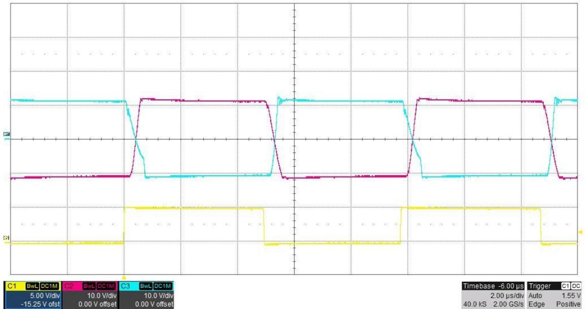
The photo below shows the switch node voltages of **15V#1** and **5V#1**, measured at TP4 and TP12 and the PHASE clock signal. **V<sub>in</sub> = 26.4V**, **I<sub>out</sub> = 0A**. (PHASE is 5V/DIV, 10V/DIV, 2uS/DIV)
