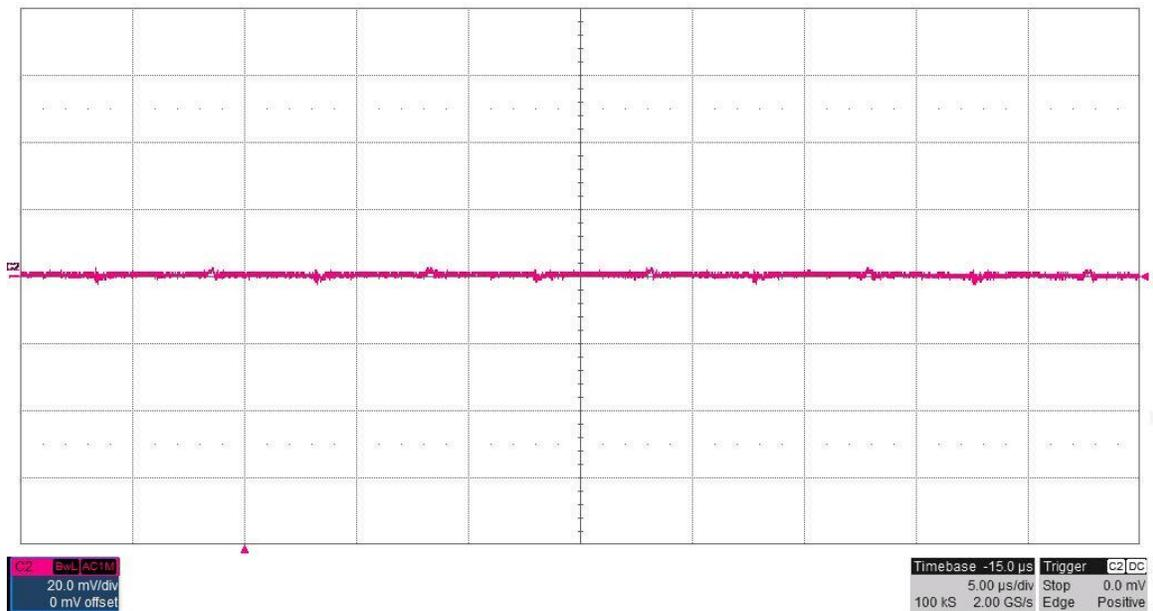
The output ripple voltage is shown in the figure below. The image was taken with the **5V#2** output loaded to **0.15A** and the input voltage set to 26.4V. (20mV/DIV, 5uS/DIV)
