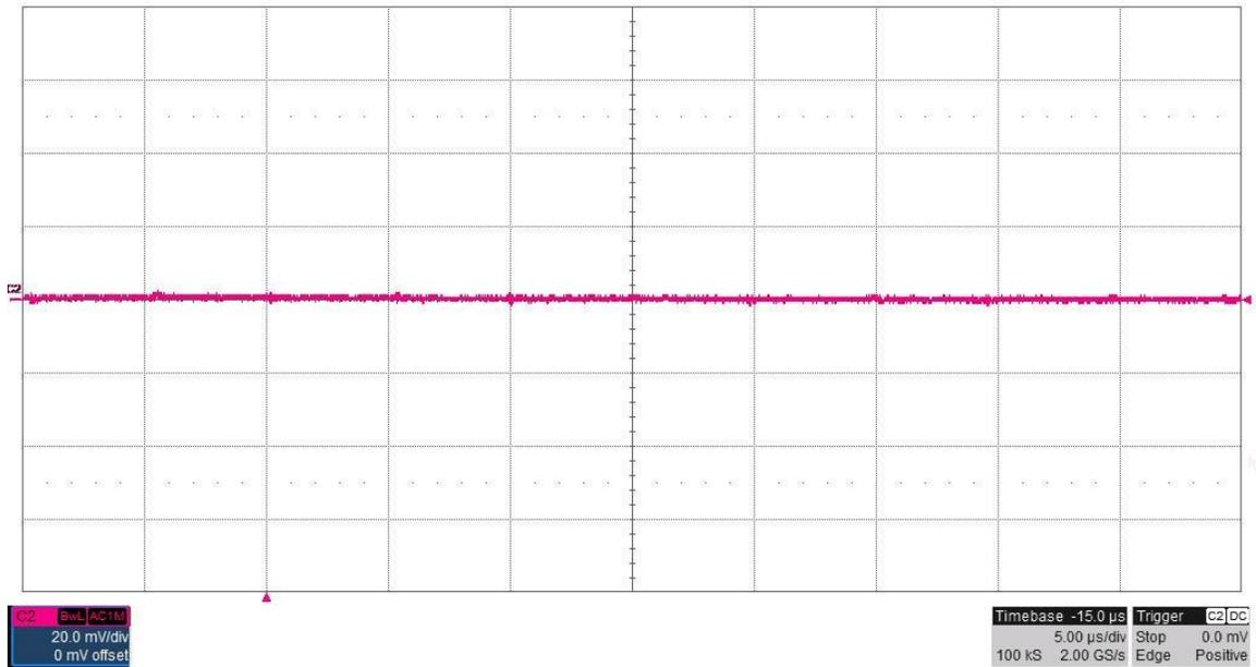
The output ripple voltage is shown in the figure below. The image was taken with the **15V#2** output loaded to **0.15A** and the input voltage set to 26.4V. (20mV/DIV, 5uS/DIV)
