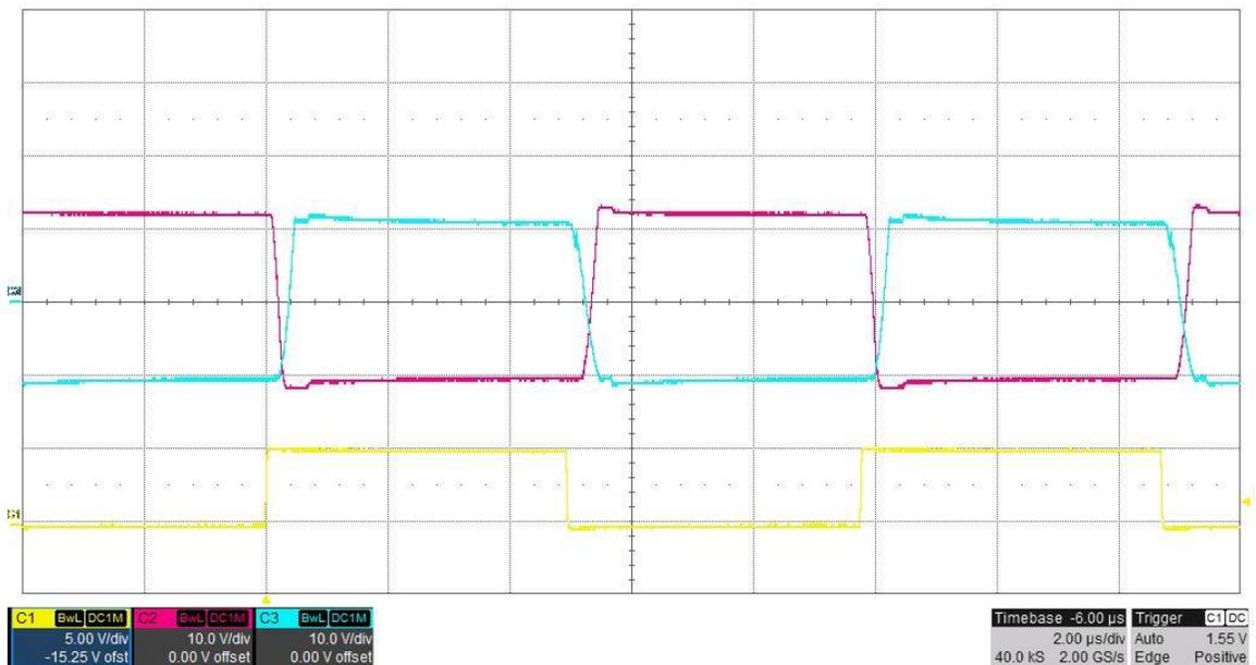
The photo below shows the switch node voltages of **15V#2** and **5V#2**, measured at TP18 and TP25 and the PHASE clock signal. **V<sub>in</sub> = 26.4V**, **I<sub>out</sub> = 0A**. (PHASE is 5V/DIV, 10V/DIV, 2uS/DIV)
