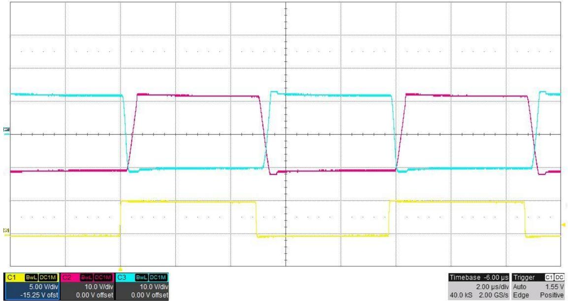
The photo below shows the switch node voltages of **15V#1** and **5V#1**, measured at TP4 and TP12 and the PHASE clock signal. **V<sub>in</sub> = 21.6V**, **I<sub>out</sub> = 0.15A**. (PHASE is 5V/DIV, 10V/DIV, 2uS/DIV)
