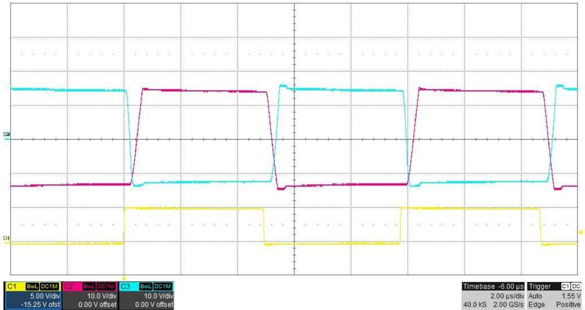
The photo below shows the switch node voltages of **15V#1** and **5V#1**, measured at TP4 and TP12 and the PHASE clock signal. **V<sub>in</sub> = 26.4V**, **I<sub>out</sub> = 0.15A**. (PHASE is 5V/DIV, 10V/DIV, 2uS/DIV)
