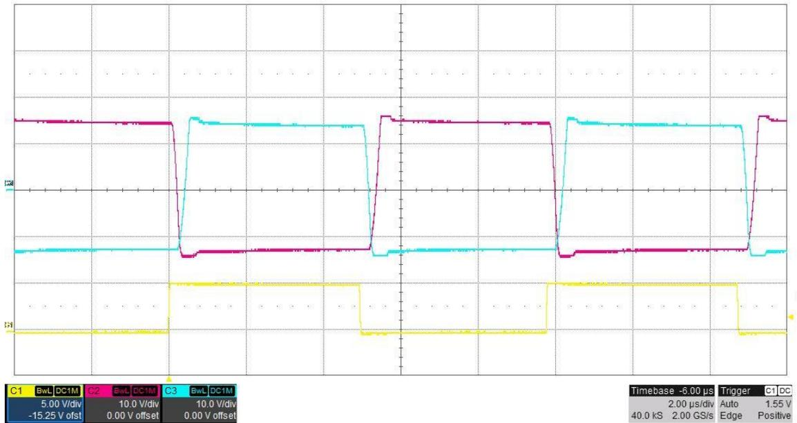
The photo below shows the switch node voltages of **15V#2** and **5V#2**, measured at TP18 and TP25 and the PHASE clock signal. **V<sub>in</sub> = 26.4V**, **I<sub>out</sub> = 0.15A**. (PHASE is 5V/DIV, 10V/DIV, 2uS/DIV)
