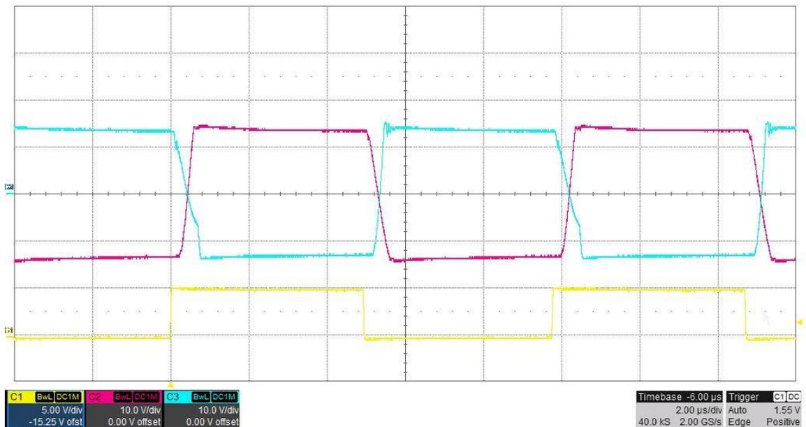
The photo below shows the switch node voltages of **15V#2** and **5V#2**, measured at TP18 and TP25 and the PHASE clock signal. **V<sub>in</sub> = 21.6V**, **I<sub>out</sub> = 0A**. (PHASE is 5V/DIV, 10V/DIV, 2uS/DIV)
