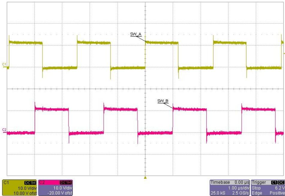
Figure 12: Switch node voltage at full 3A load on both channels, 12V input
