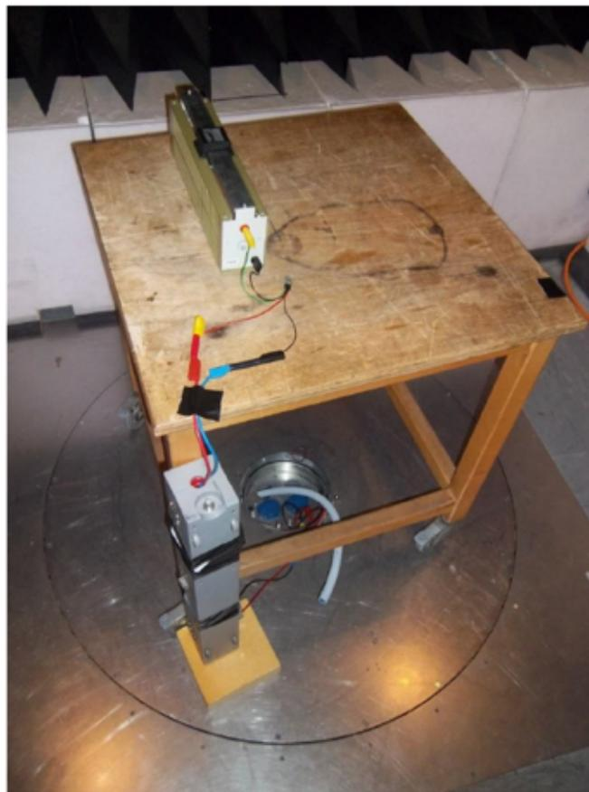
**Figure 26. Radiated Emission 3-m Prescan Test Setup**
