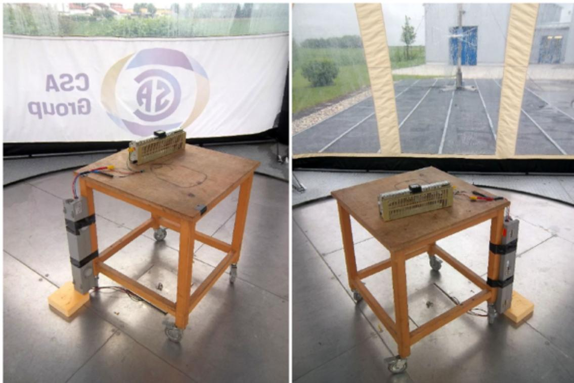
**Figure 29. Radiated Emission 10-m Test Setup**
