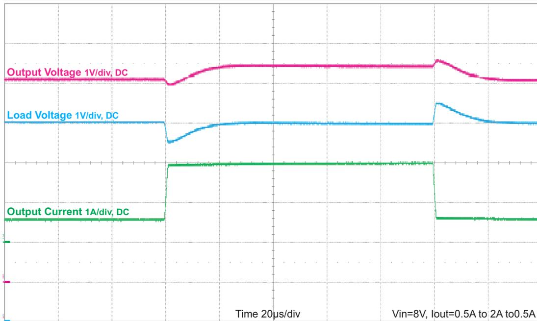
**Figure 7. Load Transient**
