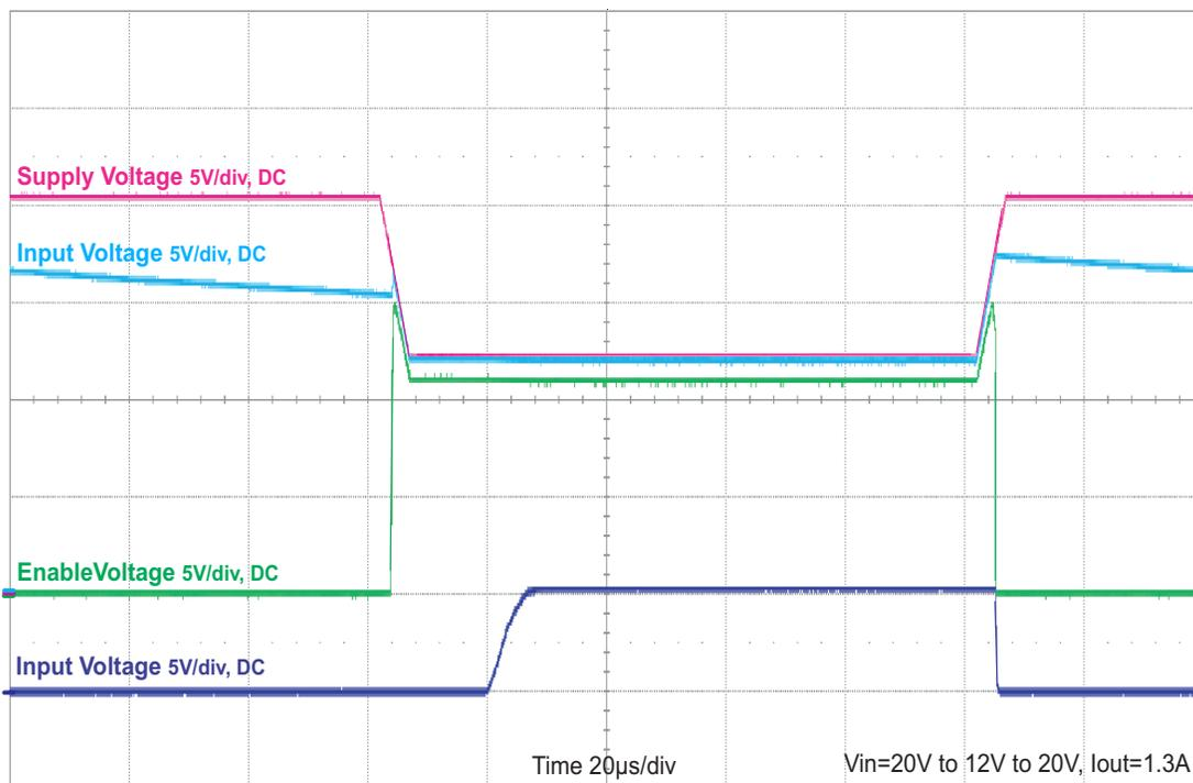
Figure 4. Overvoltage Protection
