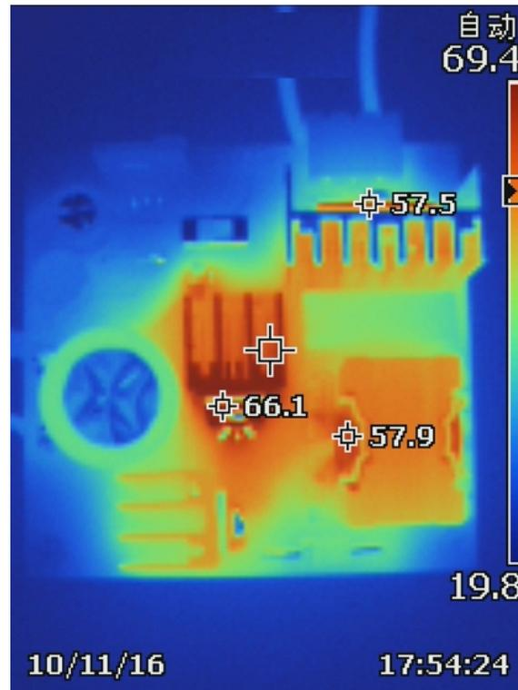
Figure 27. Top-Side Thermal Image of Converter PCB at 230-V AC Input and 350-W Load
