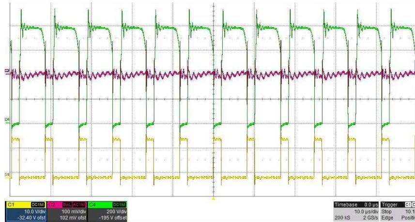
Figure 26. Switch Node and Gate Drive Waveforms Under  $V_{IN} = 600\text{ V}$  and  $I_{OUT} = 4\text{ A}$  (With Optocoupler)
