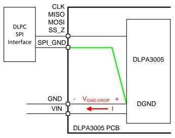
Figure 14. SPI Connections
