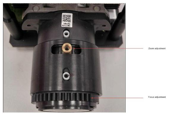
Figure 6. Optical Module With Focus and Zoom Adjustment
