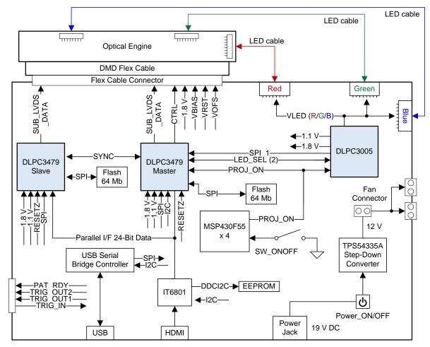
Figure 2. TIDA-080005 Block Diagram
