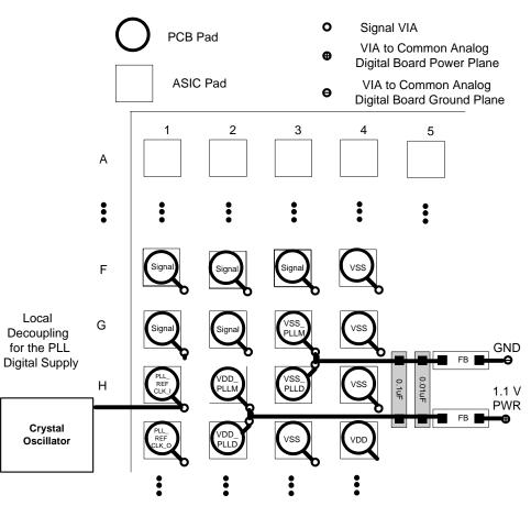
Figure 12. PLL Filter Layout
