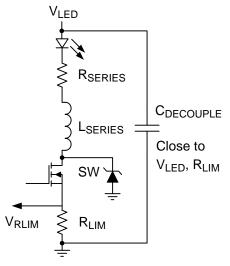
Figure 15. Parasitic Inductance (L<sub>Series</sub>) and Resistance (R<sub>series</sub>) in Series with LED
