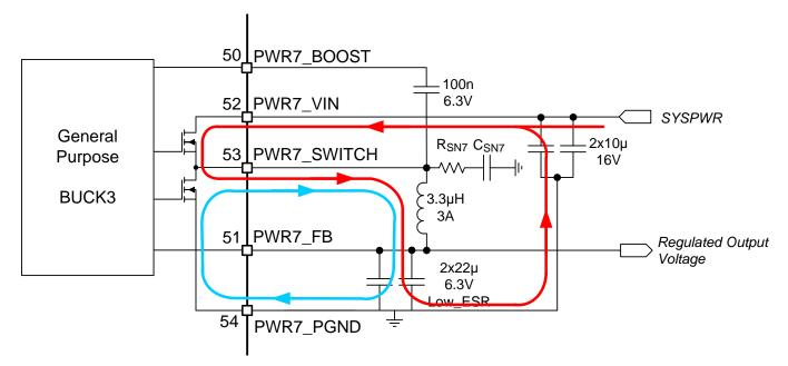
Figure 13. High AC Current Paths in a Buck Converter
