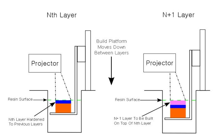
Figure 3. Top-Down 3D Printing Method
