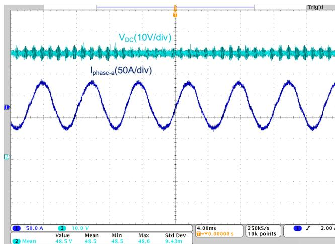
**Figure 4-6. DC Bus Voltage and Phase Current Waveforms at Motor Speed = 2000 rpm, Current Reference = 55 A**
