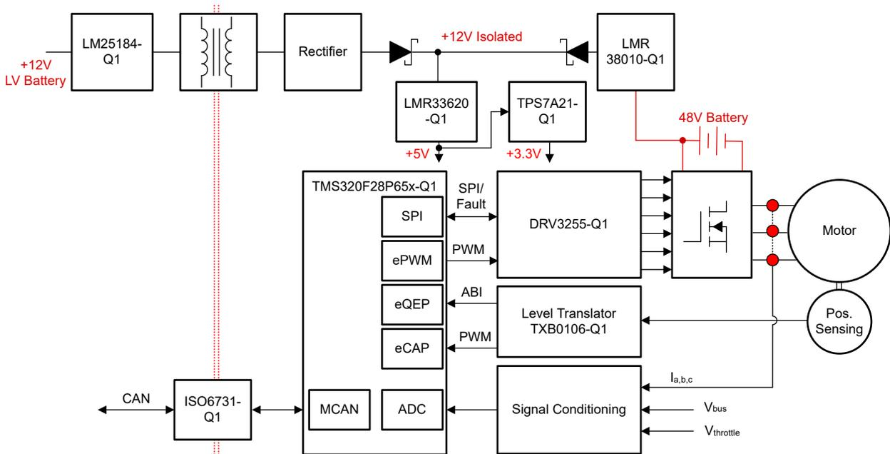
**Figure 4-1. TIDM-02017 Hardware Board Block Diagram**
