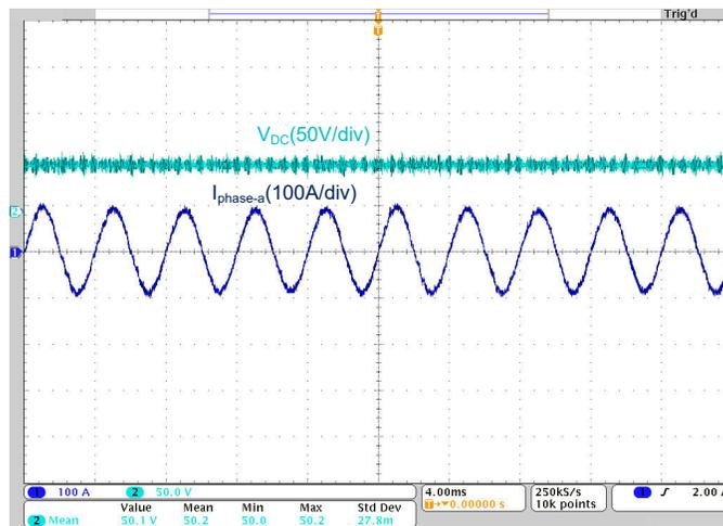
Figure 4-8. DC Bus Voltage and Phase Current Waveforms at Motor Speed = 3000 rpm, Current Reference = 95 A
