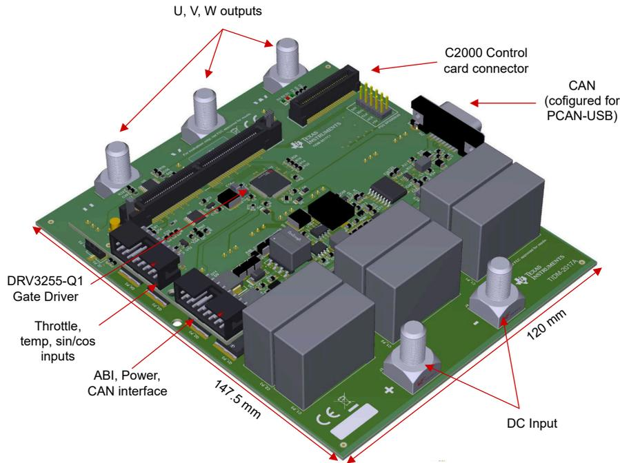
**Figure 4-2. Layout of Two-Wheeler Traction Inverter Reference Design Board**
