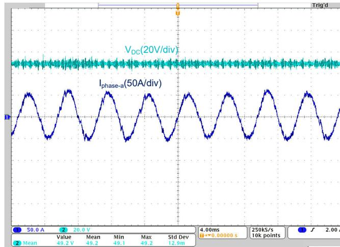
Figure 4-7. DC Bus Voltage and Phase Current Waveforms at Motor Speed = 2500 rpm, Current Reference = 55 A
