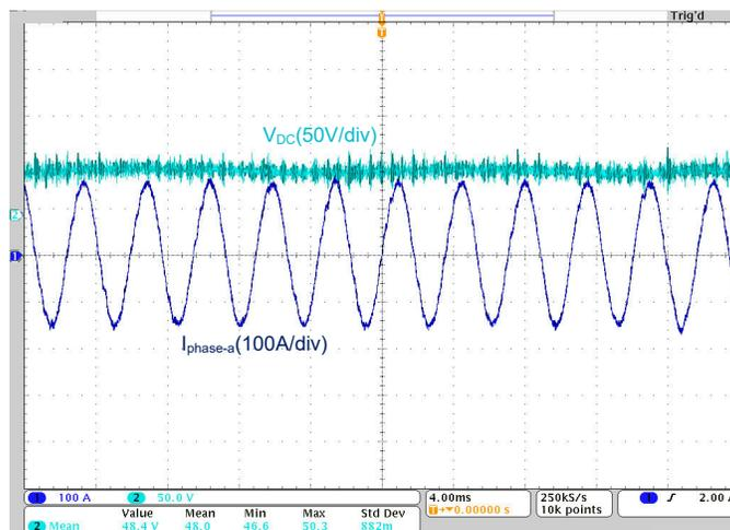
Figure 4-9. DC Bus Voltage and Phase Current Waveforms at Motor Speed = 3500 rpm, Current Reference = 160 A
