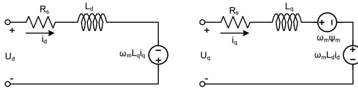
**Figure 3-8. Equivalent Circuit of an IPM Synchronous Motor**
