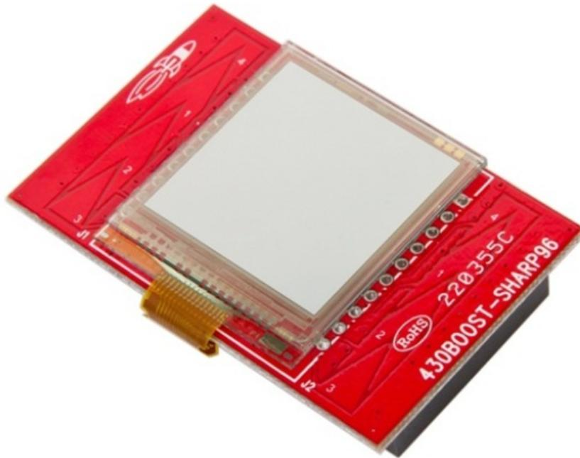
Figure 8. 430BOOST-SHARP96 Graphics LCD BoosterPack
