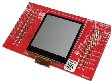
Figure 9. BOOSTXL-SHARP128 Graphics LCD BoosterPack
