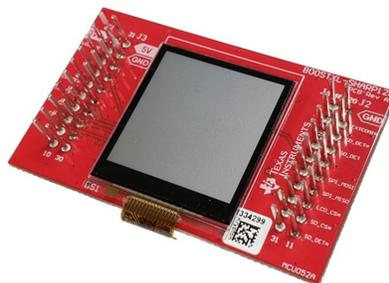
Figure 9. BOOSTXL-SHARP128 Graphics LCD BoosterPack
