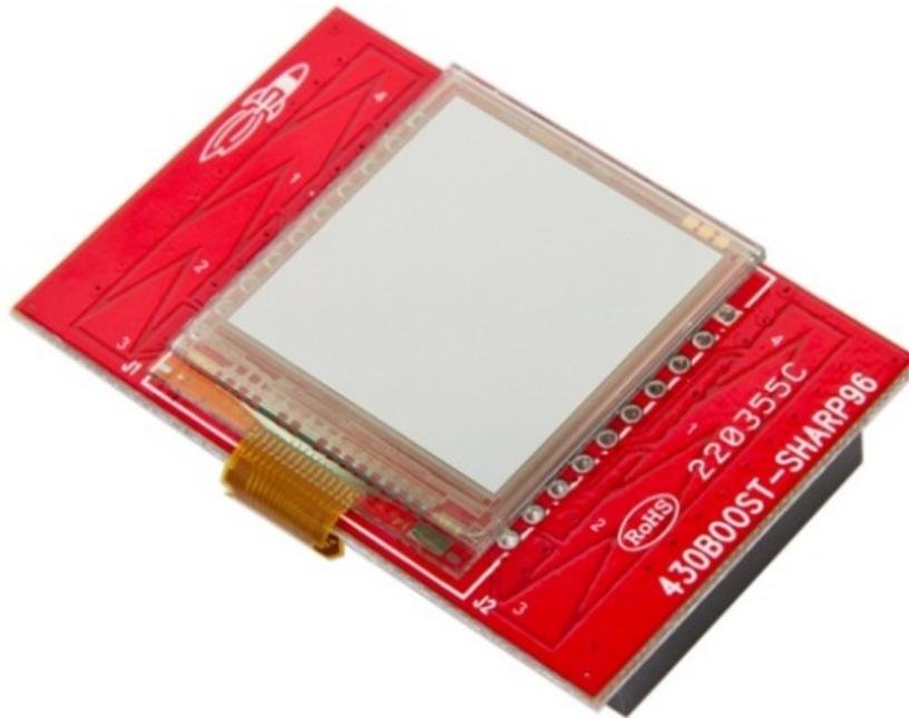
Figure 8. 430BOOST-SHARP96 Graphics LCD BoosterPack
