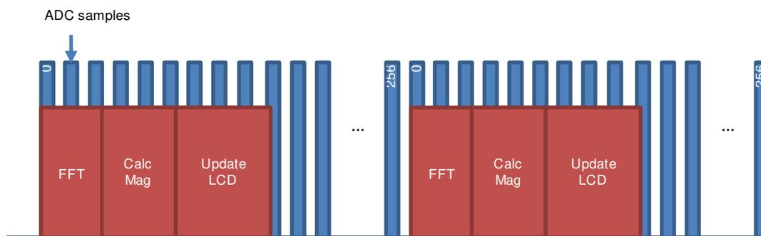
Figure 3. Generic Timing Diagram for FFT Operation
