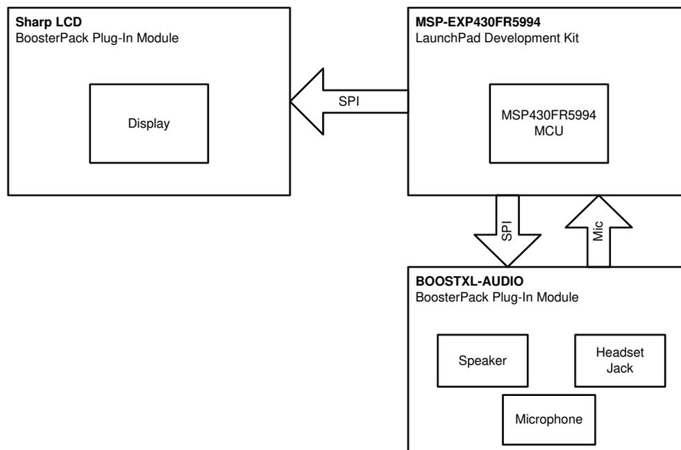
Figure 1. Block Diagram Theory
