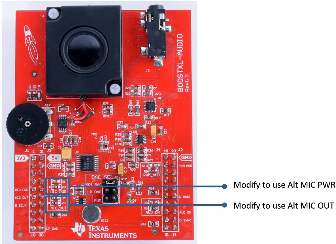
Figure 7. BOOSTXL-AUDIO BoosterPack Required Modification
