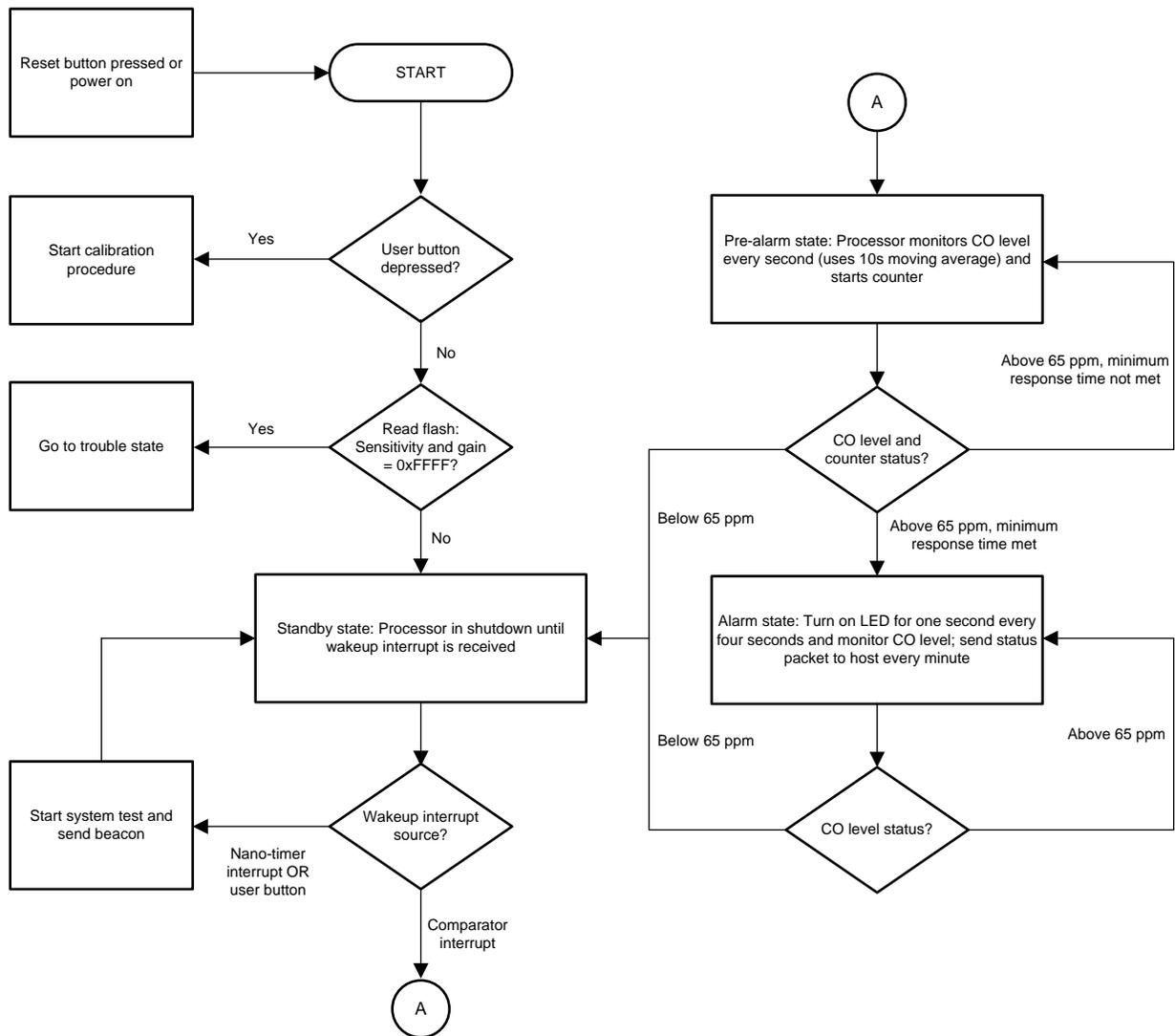
Figure 13. Normal Operation Flowchart
