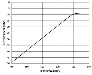
Figure 17. ICS-40300 dBV Output Curve
