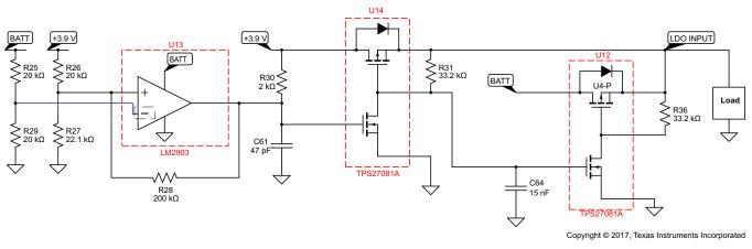
Figure 12. TIDA-01519 ORing Circuit
