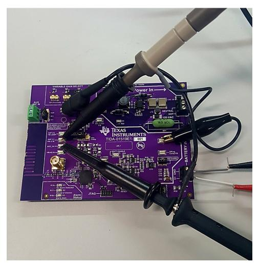
Figure 46. Setup of Audio Response Probe
