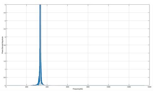
Figure 38. Power Spectral Density Plot of 3-kHz Alarm at 10-ft Proximity
