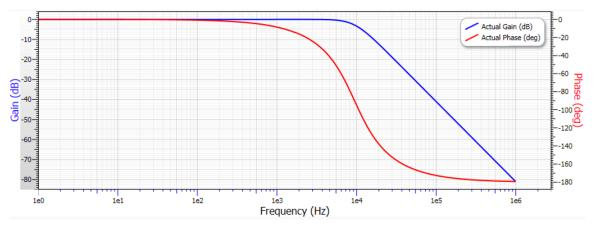
Figure 25. TIDA-01519 Antialiasing Filter Frequency Response Plot
