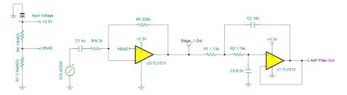
Figure 27. TIDA-01519 Signal Chain Simulation Schematic
