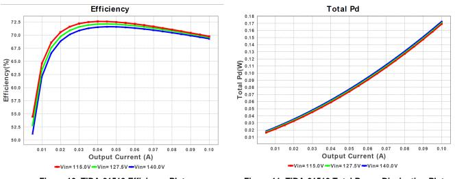
Figure 10. TIDA-01519 Efficiency Plot
