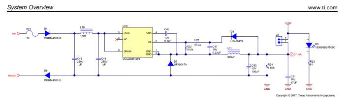
Figure 9. TIDA-01519 120-V AC to DC Schematic
