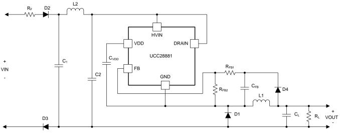
Figure 8. 120-V AC to DC Conversion Circuit, 3.9-V and 100-mA Output
