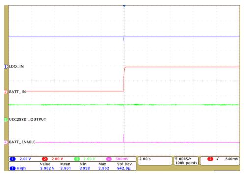
Figure 58. UCC28881 Power on With Battery Applied as Secondary Power Source
