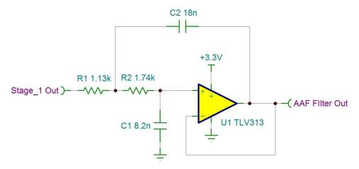
Figure 24. TIDA-01519 Antialiasing Filter Circuit
