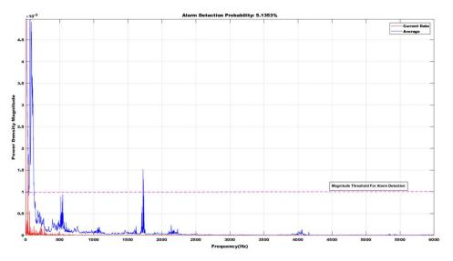
Figure 54. 24-Hour Proximity Averaged Spectral Power Density Response
