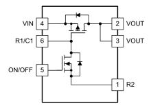
Figure 6. TPS27081A Functional Block Diagram
