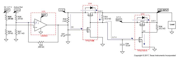
Figure 13. ORing: UCC28881 Primary Power Circuit Logic
