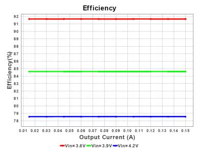
Figure 16. TPS780330220 Efficiency Curve Plot
