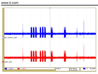
Figure 52. Signal Chain Response at 10-ft Proximity
