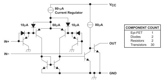
Figure 7. LM2903DGKR Functional Block Diagram
