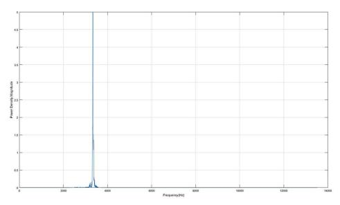
Figure 37. Power Spectral Density Plot of 3-kHz Alarm at 2-ft Proximity
