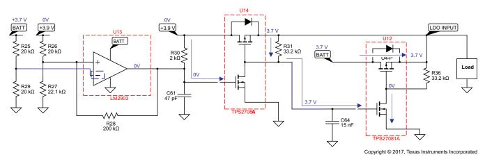
Figure 14. ORing: Battery Primary Power Circuit Logic
