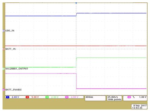
Figure 57. Test Results of Power ORing
