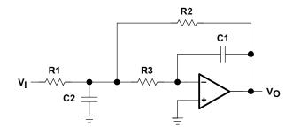
Figure 23. Second-Order Unity Gain Sallen-Key Low-Pass Filter Topology
