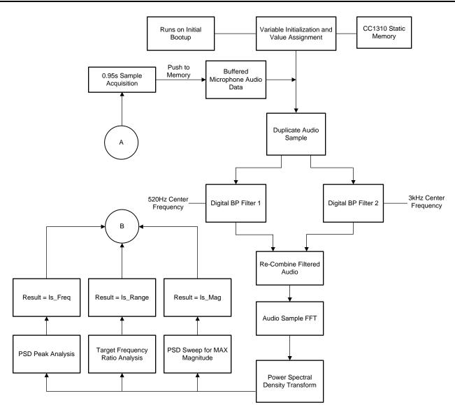
Figure 39. TIDA-01519 Audio Processing Flow Chart
