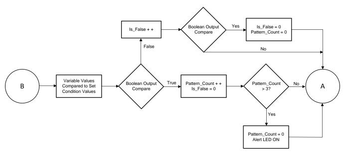
Figure 40. TIDA-01519 Alarm Detection Algorithm Software Flow Chart
