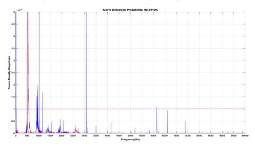
Figure 55. 520 Hz at 5-ft Proximity Alarm Detected Spectral Power Density Response
