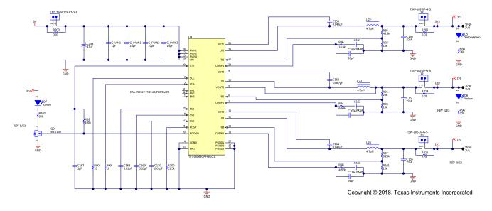
Figure 10. TPS65263 Multi-Rail Converter Stage
