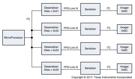
Figure 4. I<sup>2</sup>C Address Aliasing
