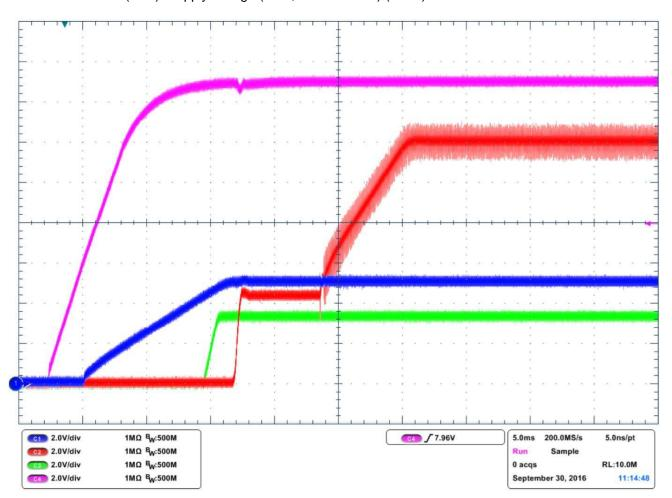
Figure 12. Power Supply Startup Waveform
