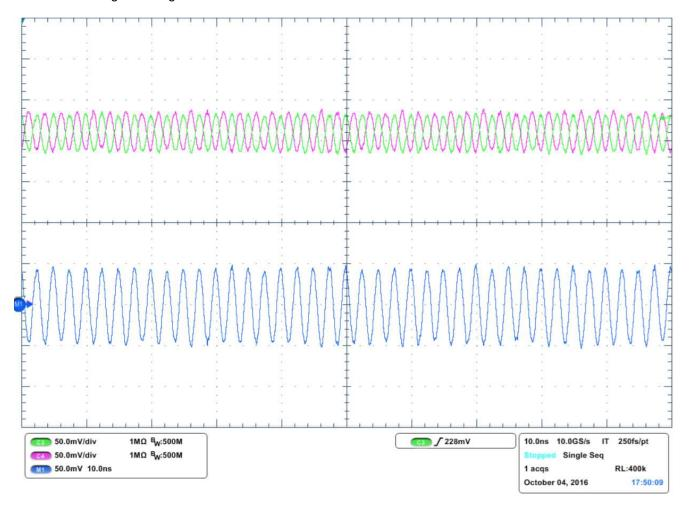
Figure 16. CSI-2 Positive and Negative Differential Voltages Measured
