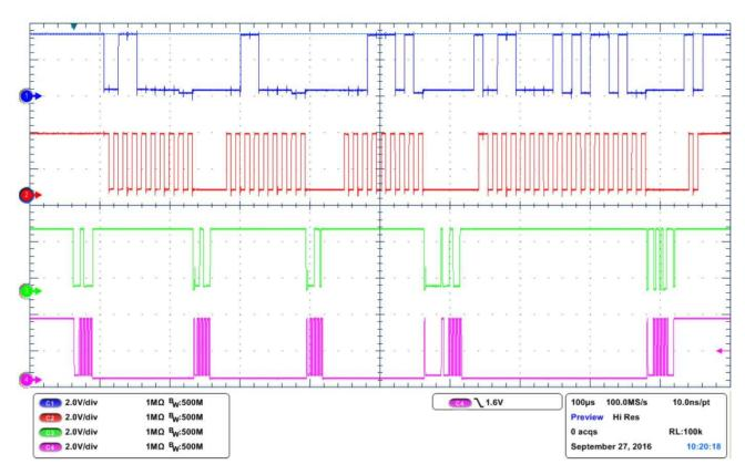
Figure 13. I<sup>2</sup>C Communication Waveforms
