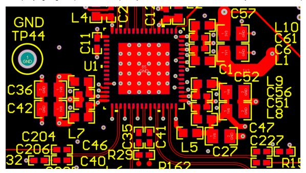
Figure 19. FPD-Link Input, MIPI CSI-2 Differential Pairs, and Decoupling Current Loop
