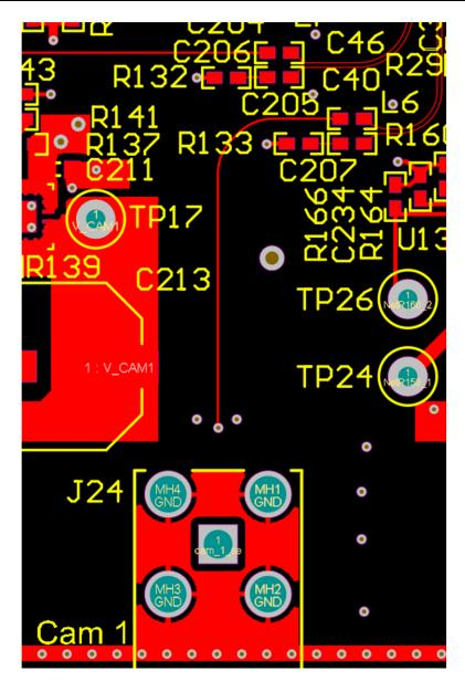
Figure 20. LVDS Signal Pair Routing
