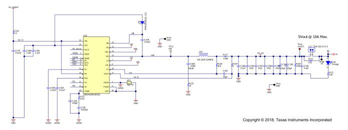
Figure 8. LM5141 Buck Converter Stage
