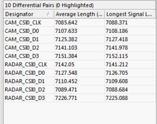
Figure 22. CSI-2 Differential Trace Routing
