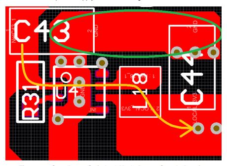
Figure 18. Step-Down Switched-Mode Power Supply Routing
