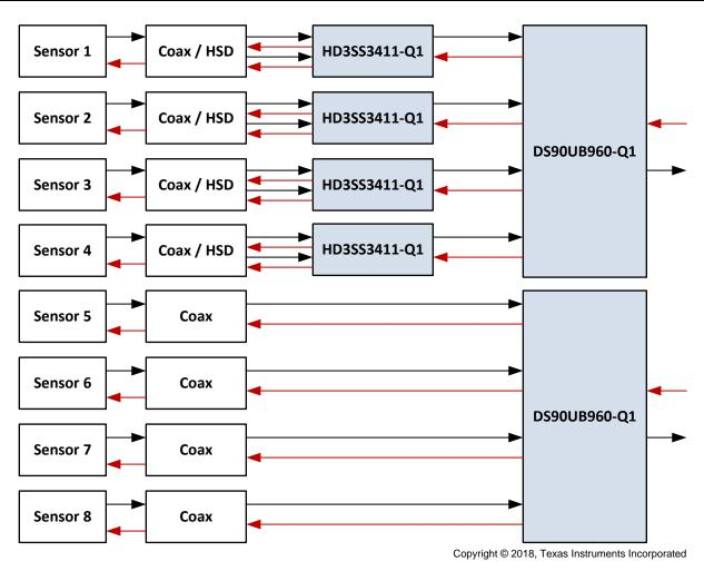
Figure 6. Coax vs HSD Connection Setup
