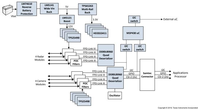
Figure 1. TIDA-01413 Block Diagram
