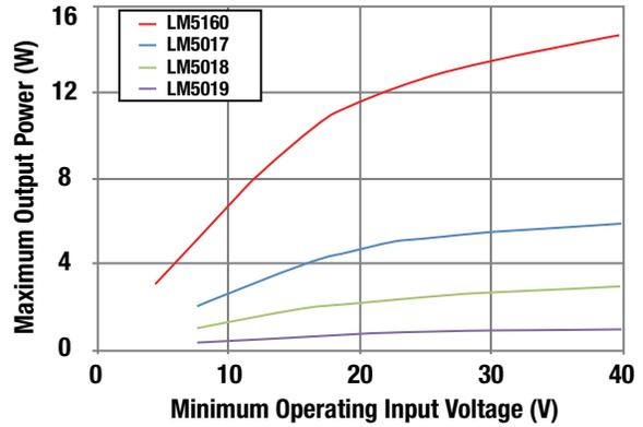
Figure 9. Maximum output power of Fly-Buck converters
