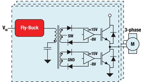
Figure 2. IGBT/SiC/MOSFET gate drive bias rails
