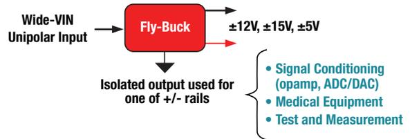
Figure 4. Bipolar ( $\pm$ ) rails for instrumentation
