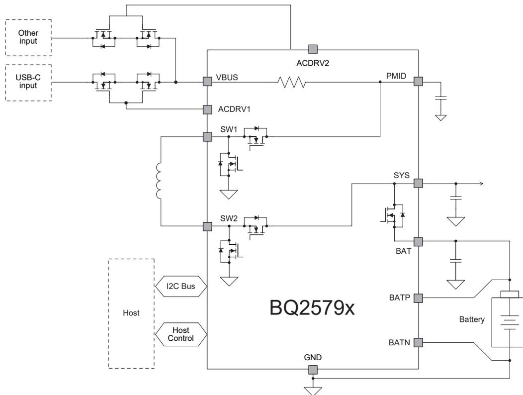
Figure 2. Example of a fully integrated buck-boost charger.
