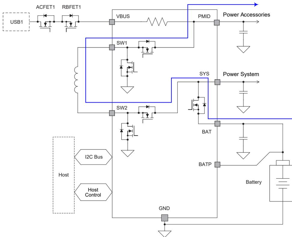
**Figure 3.** USB Type-C™ FRS realized by single buck-boost charger.
