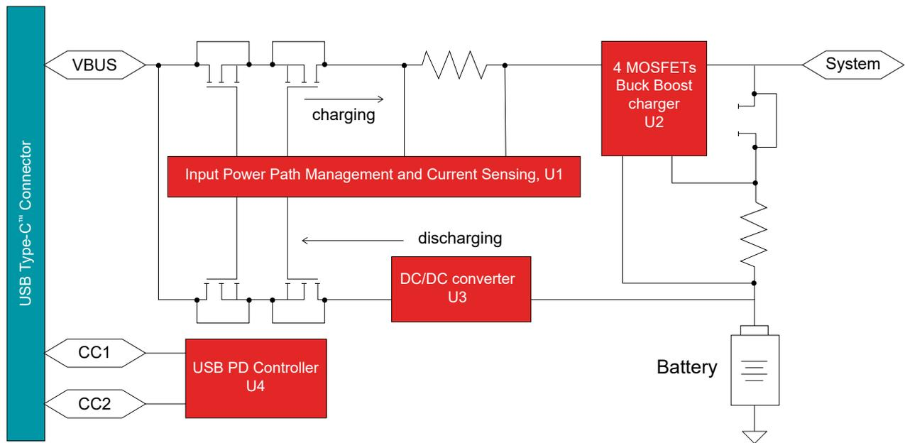
**Figure 1.** Block diagram for a USB PD charging solution.
