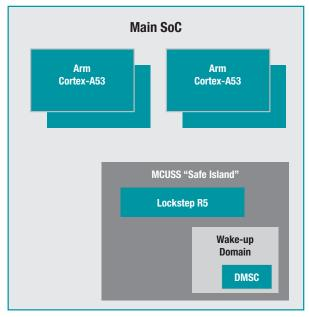
Figure 6: MCUSS in the AM6x processor.
