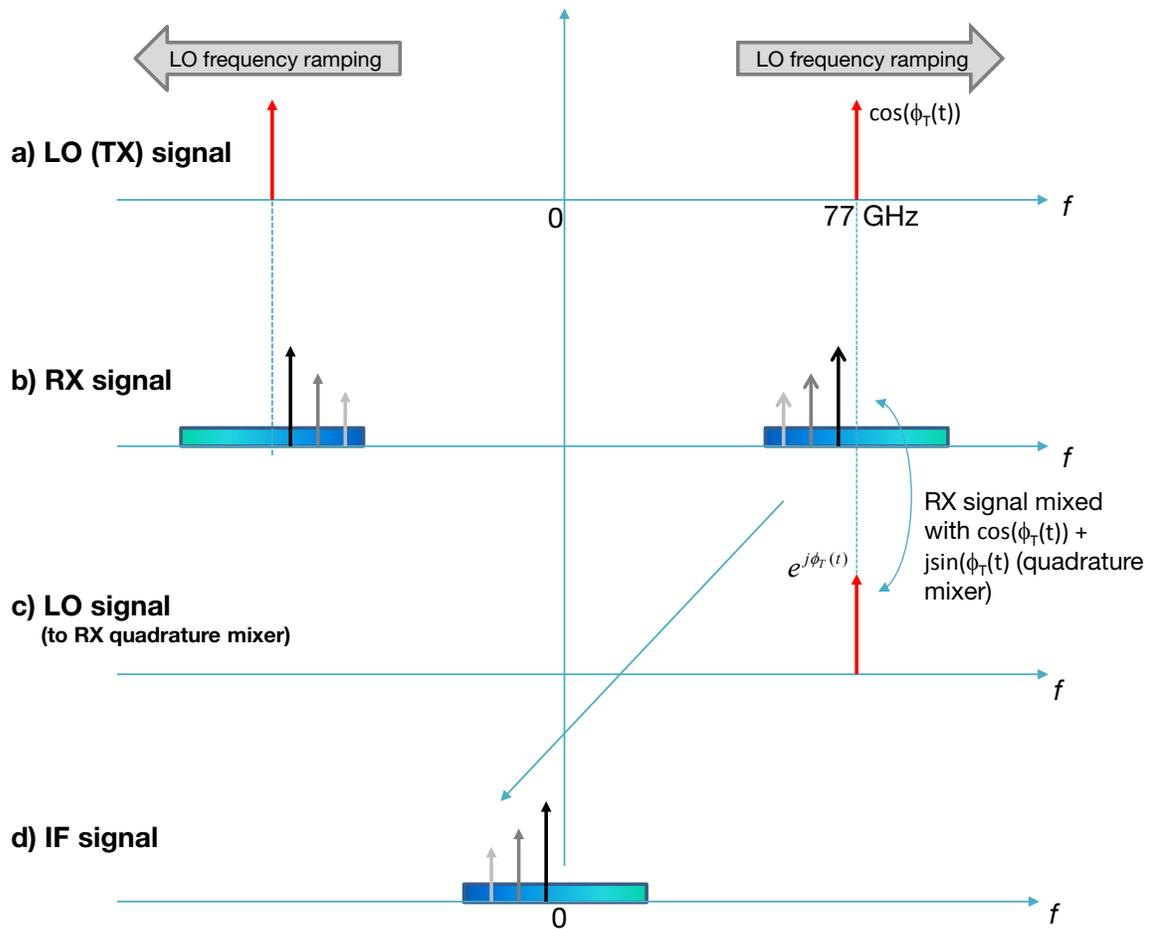
**Figure 6.** Quadrature mixer and complex baseband with no image-band noise foldback. (a) Instantaneous spectrum of LO (TX) signal showing ramping frequency, (b) RX signal after reflection from various objects, (c) Quadrature LO signal, (d) IF signal after quadrature mixer.
