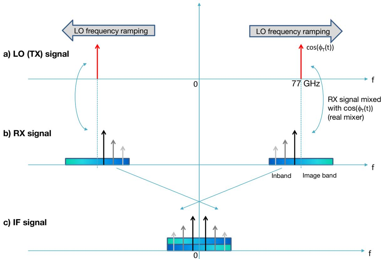
**Figure 4.** A real mixer and real baseband suffers from image-band noise foldback. (a) Instantaneous spectrum of LO (TX) signal showing ramping frequency, (b) RX signal after reflection from various objects, (c) IF signal after real mixer.
