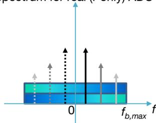
Spectrum for complex (I,Q) ADC output
