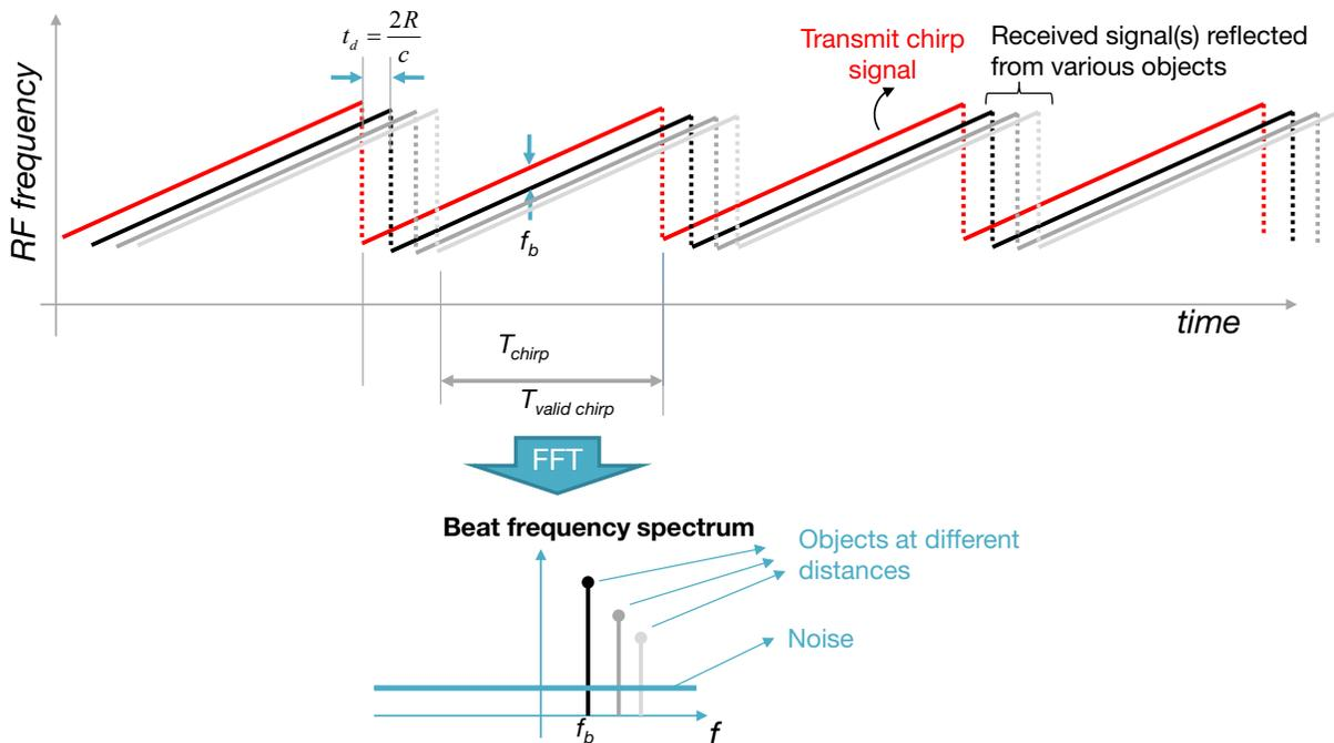
Figure 3. Received FMCW radar signal and beat-frequency spectrum.
