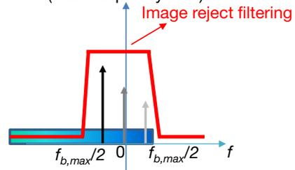
Figure 8. Beat-frequency spectrum for real and complex-baseband outputs.
