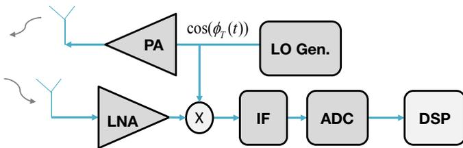
Figure 2. High-level block diagram of an FMCW radar.
