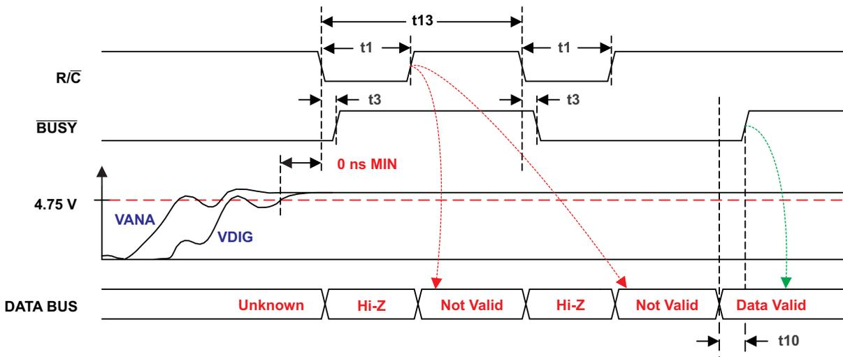
Figure 1. ADS8504/05 NEW SAR Reset Function
