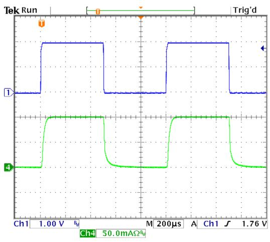
Figure 13. Full-Scale Settling Response
