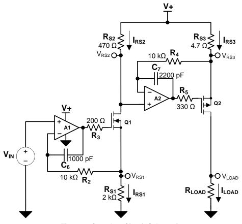
Figure 2. Complete Circuit Schematic
