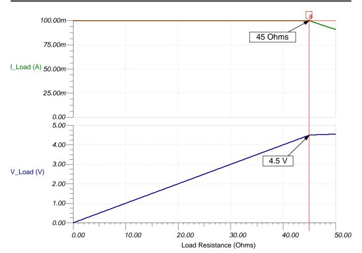
Figure 7. TINA-TI<sup>™</sup> - Compliance Voltage and Maximum Load Resistance
