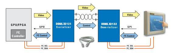
Figure 4. Display Application, 21-Bit LVCMOS Bus and Embedded I<sup>2</sup>C Compatible Control
