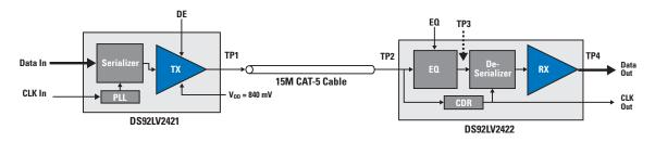
Figure 2. Channel Link II SerDes I/O Block Diagram and Test Case
