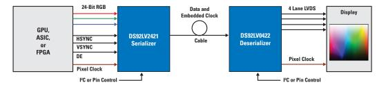
Figure 5. Format Conversion with Channel Link II and III SerDes
