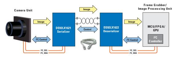
Figure 3. Camera Application, 16-Bit LVCMOS Bus and Embedded I<sup>2</sup>C Compatible Control
