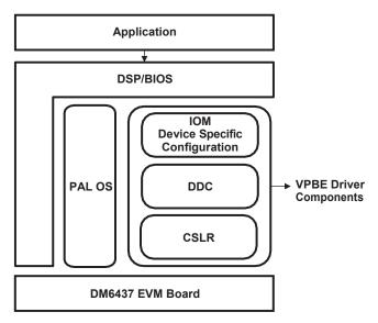
Figure 2. VPBE Driver Structure
