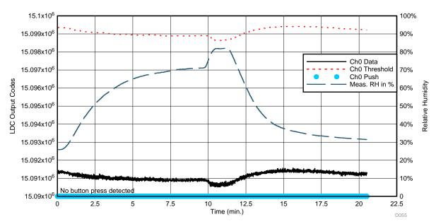
Figure 50. LDC Ch0 Data During Relative Humidity "Shock" Test—Down Button Channel
