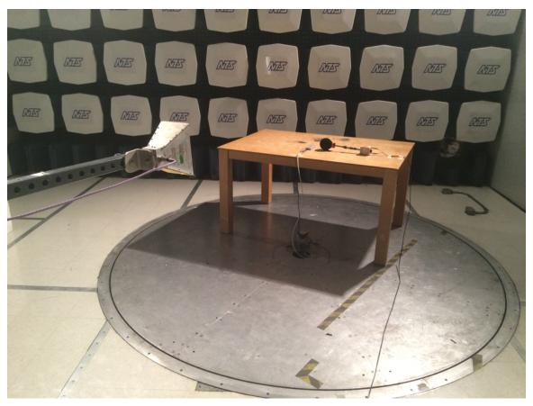
Figure 55. IEC 61000-4-3 Radiated Immunity Test Setup
