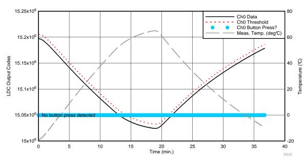
Figure 45. LDC Ch0 Data During Thermal "Shock" Test—Down Button Channel
