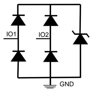
Figure 12. TPD2E2U06 Functional Block Diagram
