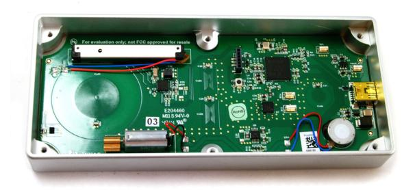
Figure 14. Touch on Metal Buttons With Integrated Haptic Feedback Reference Design Hardware
