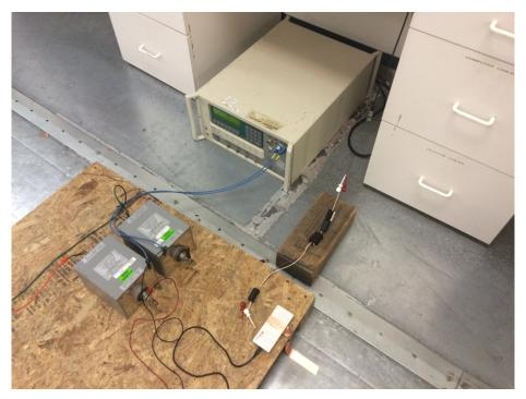
Figure 74. IEC 61000-4-5 Surge Test Setup
