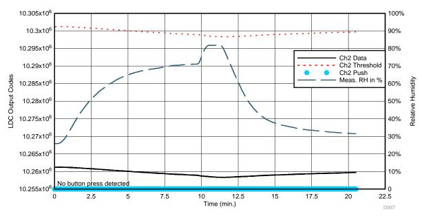
Figure 52. LDC Ch2 Data During Relative Humidity "Shock" Test—Big Button Channel
