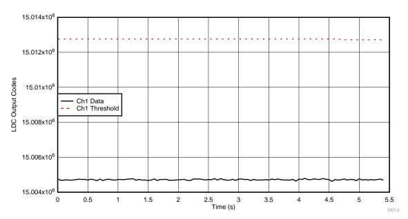
Figure 36. LDC Ch1 Data During LRA Activation—Up Button Channel
