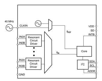
Figure 5. LDC1614 Functional Block Diagram
