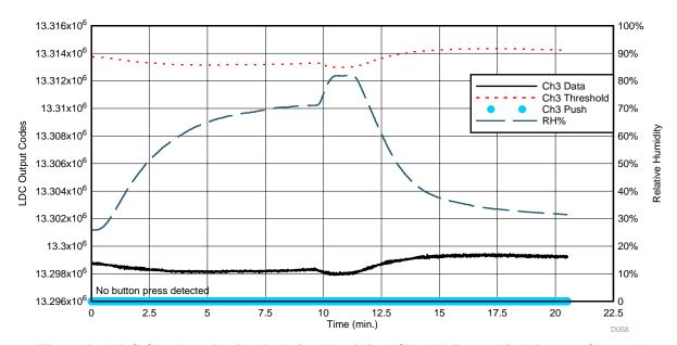
Figure 53. LDC Ch3 Data During Relative Humidity "Shock" Test—Little Button Channel
