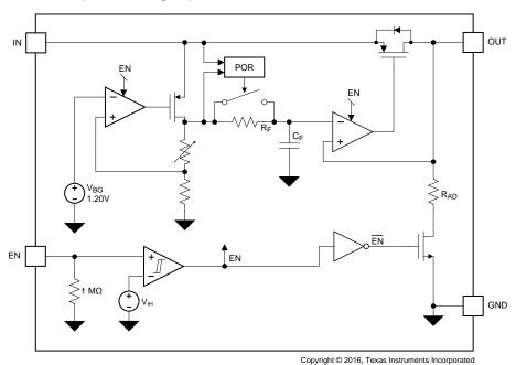
Figure 10. LP5907 Functional Block Diagram
