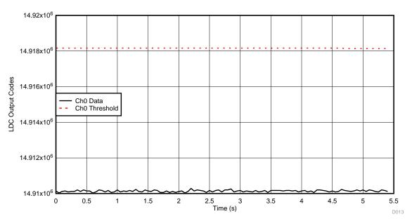
Figure 35. LDC Ch0 Data During LRA Activation—Down Button Channel
