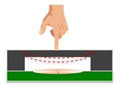
Figure 1. Mechanical Deflection Detail
