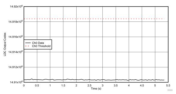
Figure 31. LDC Ch0 Data During ERM Activation—Down Button Channel
