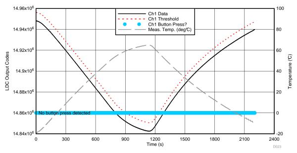
Figure 46. LDC Ch1 Data During Thermal "Shock" Test-Up Button Channel
