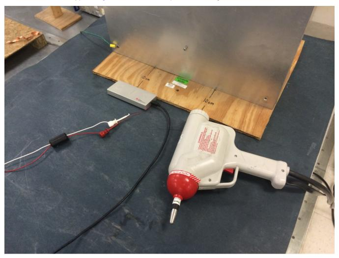
Figure 54. IEC 61000-4-2 ESD Test Setup
