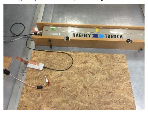
Figure 73. IEC 61000-4-4 EFT Test Setup
