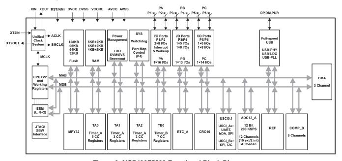
Figure 9. MSP430F5528 Functional Block Diagram
