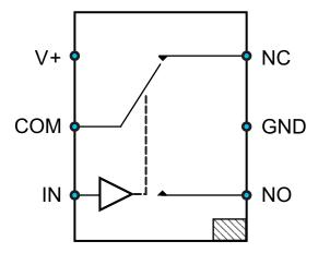
Figure 11. TS5A12301E Logic Diagram
