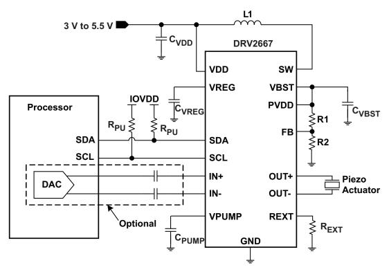
Figure 7. DRV2667 System Diagram
