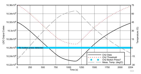
Figure 47. LDC Ch2 Data During Thermal "Shock" Test—Big Button Channel
