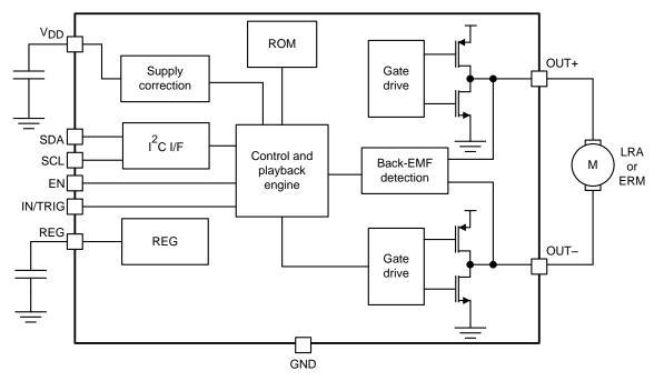
Figure 6. DRV2605L Functional Block Diagram
