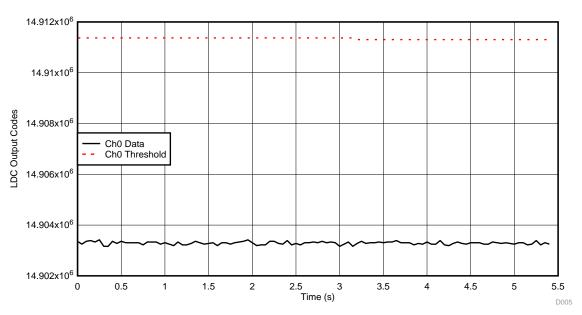
Figure 27. LDC Ch0 Data During Piezo Activation—Down Button Channel
