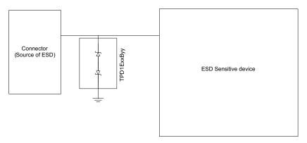
Figure 13. TPD1E10B06 Device Configuration
