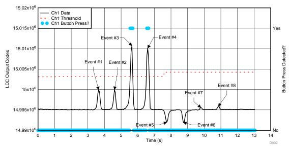
Figure 19. LDC Ch1 Data—Up Button Channel
