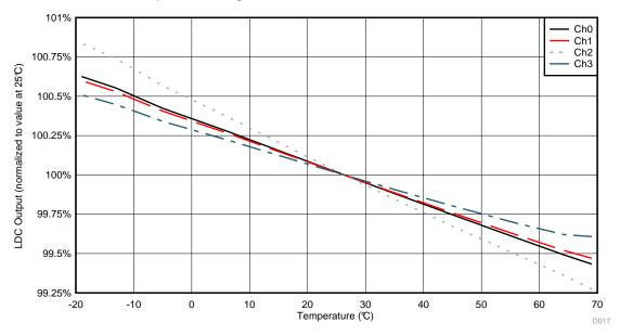
Figure 44. LDC1614 Data Over Temperature—All Channels
