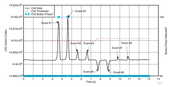
Figure 18. LDC Ch0 Data - Down Button Channel
