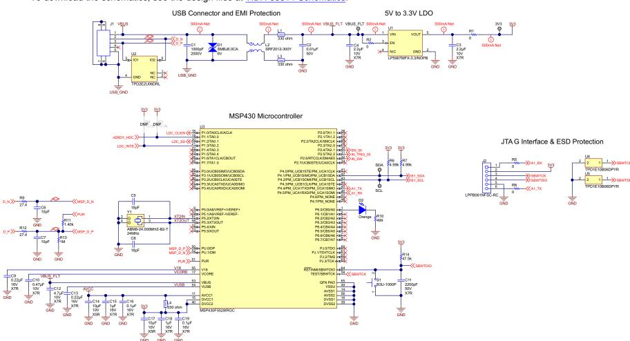
Figure 88. Touch on Metal Buttons With Integrated Haptic Feedback Schematic—Page 1
