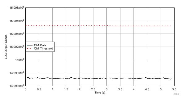
Figure 28. LDC Ch1 Data During Piezo Activation—Up Button Channel
