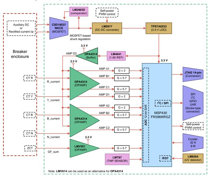
Figure 2. TIDA-00498 Block Diagram
