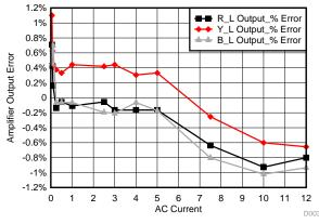
Figure 32. Current Versus Output Error for Low Gain Amplifier Using OPA4314
