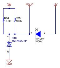
Figure 11. Comparator Power Supply Generated From 39-V Supply
