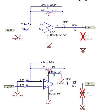
Figure 17. Amplifier With Single Gain Schematic
