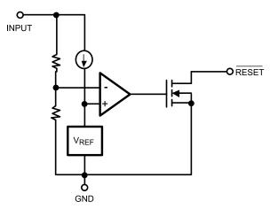
Figure 7. LM8364 Functional Block Diagram
