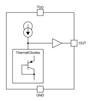
Figure 6. LMT87 Functional Block Diagram
