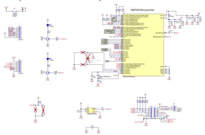
Figure 20. MCU Configuration Schematic
