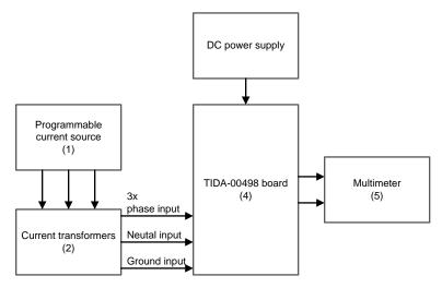
Figure 23. Test Setup Block Diagram
