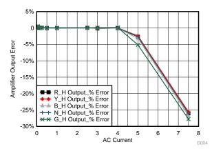
Figure 33. Current Versus Output Error for High Gain Amplifier Using OPA4314
