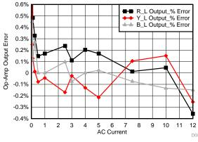
Figure 30. Current Versus Output Error for Low Gain Amplifier Using LMV614
