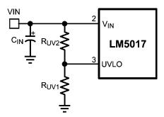
Figure 12. UVLO Resistor Setting
