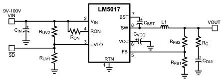
Figure 8. LM5017 Typical Application Diagram
