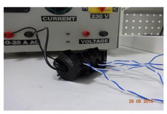
Figure 25. Current Transformer
