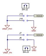
Figure 19. Jumper for AC Current or Rectified Current Schematic
