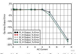
Figure 31. Current Versus Output Error for High Gain Amplifier Using LMV614
