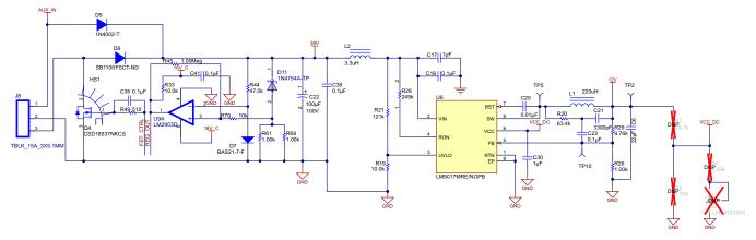
Figure 10. Self-Power Supply Including DC-DC Converter Schematic
