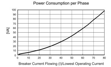
Figure 1. Typical Power Consumption for Current and Lowest Operating Current
