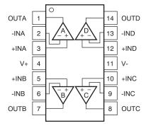
Figure 4. OPA4314 Pinout Diagram
