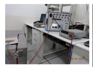
Figure 28. Temperature Chamber Setup
