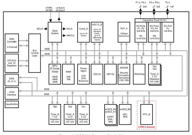
Figure 3. MSP430 System Block Diagram
