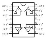
Figure 5. LMV614 Pinout Diagram
