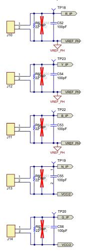
Figure 15. Current Input Connector With Burden Resistor
