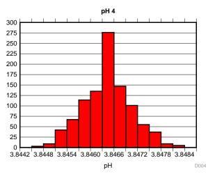
Figure 15. Measured pH When pH Buffer Equals 4
