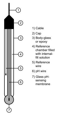
Figure 4. Typical pH Glass Electrode
