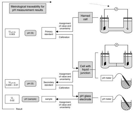
Figure 3. Metrological Traceability Scheme for pH
