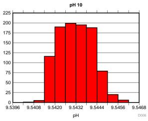
Figure 17. Measured pH When pH Buffer Equals 10
