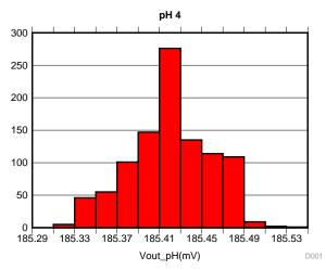
Figure 14. Measured  $V_{out}$  When pH Buffer Equals 4
