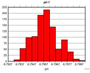
Figure 13. Measured pH When pH Buffer Equal 7
