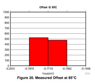
The results at room temperature are comparable to the noise performance shown in the datasheet of the ADS1120, where it says that the ENOB with PGA disabled, AVDD = 3 V, AVSS = 0 V, VREF = 2.048 (although in the TIDA-00561 there is an external reference), and the ADC is working in normal operation mode. Finally, in Figure 21,  $V_{OUT}$  in function of the temperature shows that the offset drift is equal to 0.5  $\mu$ V/°C.
