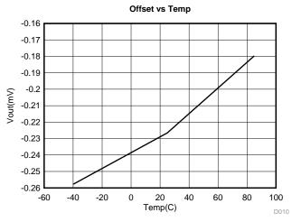
Figure 21. Offset Drift versus Temperature
