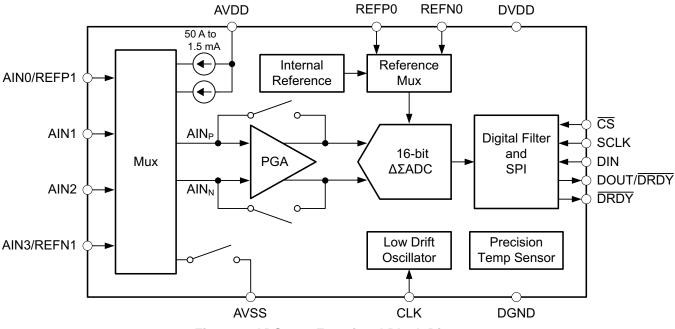
Figure 9. ADS1120 Functional Block Diagram
