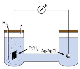
Figure 1. Harned Cell for Primary pH Measurements
