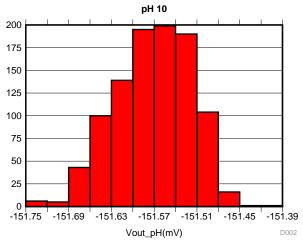
Figure 16. Measured Vout When pH Buffer Equals 10
