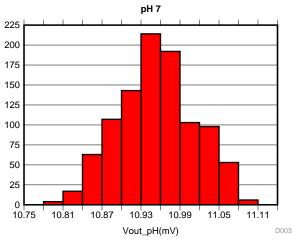
Figure 12. Measured  $V_{out}$  When pH Buffer Equals 7
