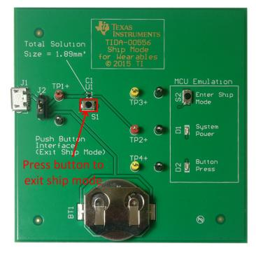
Figure 12. Configuration for Exiting Ship Mode
