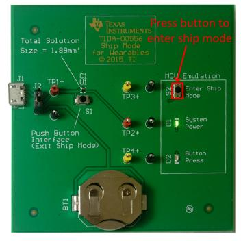
Figure 11. Configuration for Entering Ship Mode
