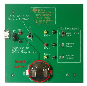
Figure 9. Ship Mode Circuit Powered Using a Battery
